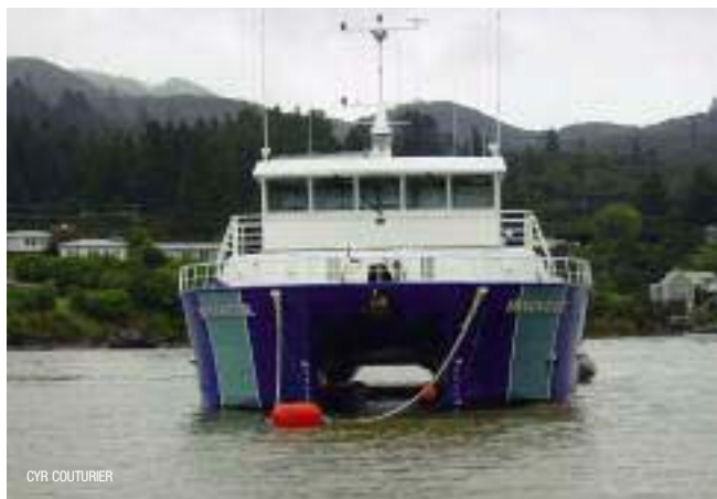
Large capacity (140 tonnes per day), ocean going mussel harvesting catamaran (35 m) used in marine mussel farming in New Zealand.
