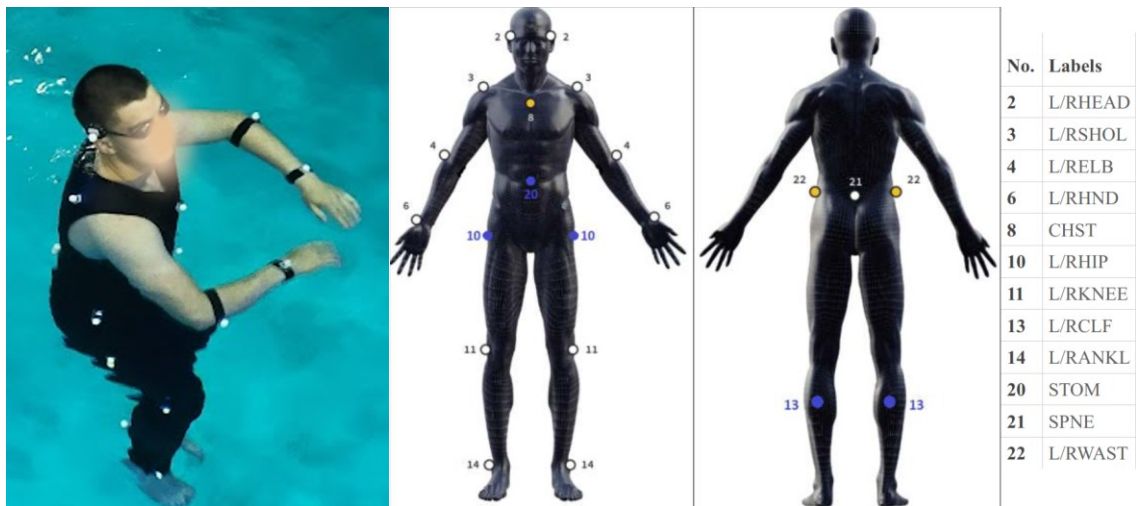
Figure 1-2: Marker set: Location of 21 passive markers and their labels.
