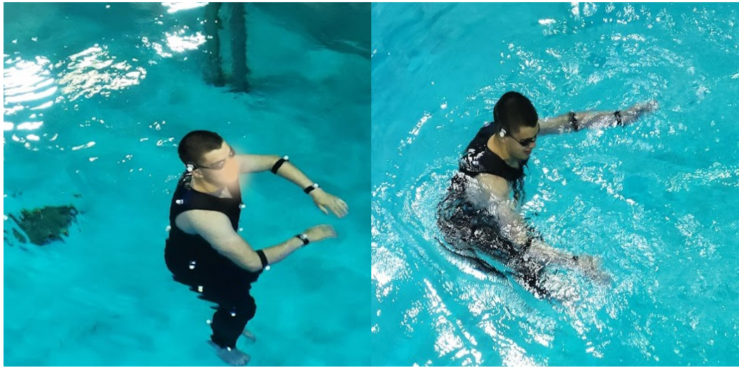
Figure 3-10: Noise in Underwater Data; Surface Reflection and Wave
