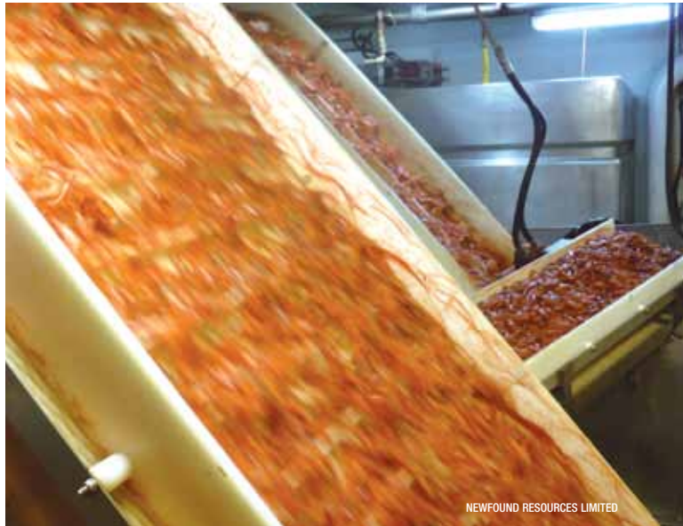
The processing of shrimp begins once the product is brought aboard the vessel. The product travels by conveyor to inspection stations, by-catch separators (pictured above), and size grading machines.
