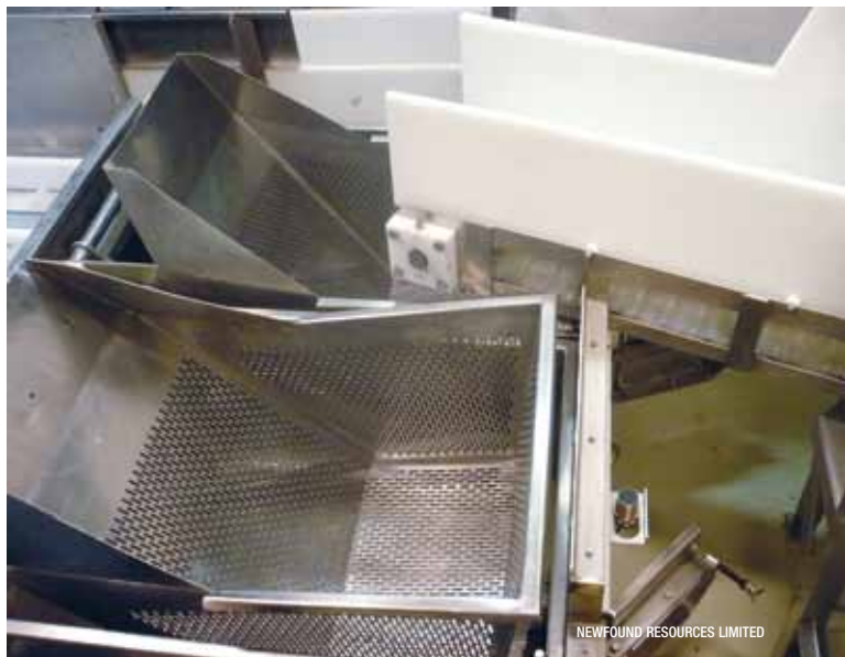
Large raw shrimp are transferred on separate conveyers to an additive treatment dip (shown above), which is a colourant and antioxidant.
