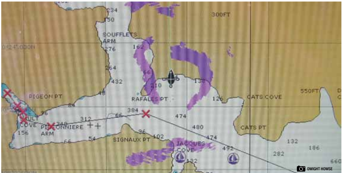
As a platform for the presentation of pertinent information for safe navigation, the electronic chart system is unparalleled. The information presented, however, is only as good as the data available in the electronic chart. Note the poor registration between the radar (purple) and the chart showing a discrepancy of about 0.75 nm.
