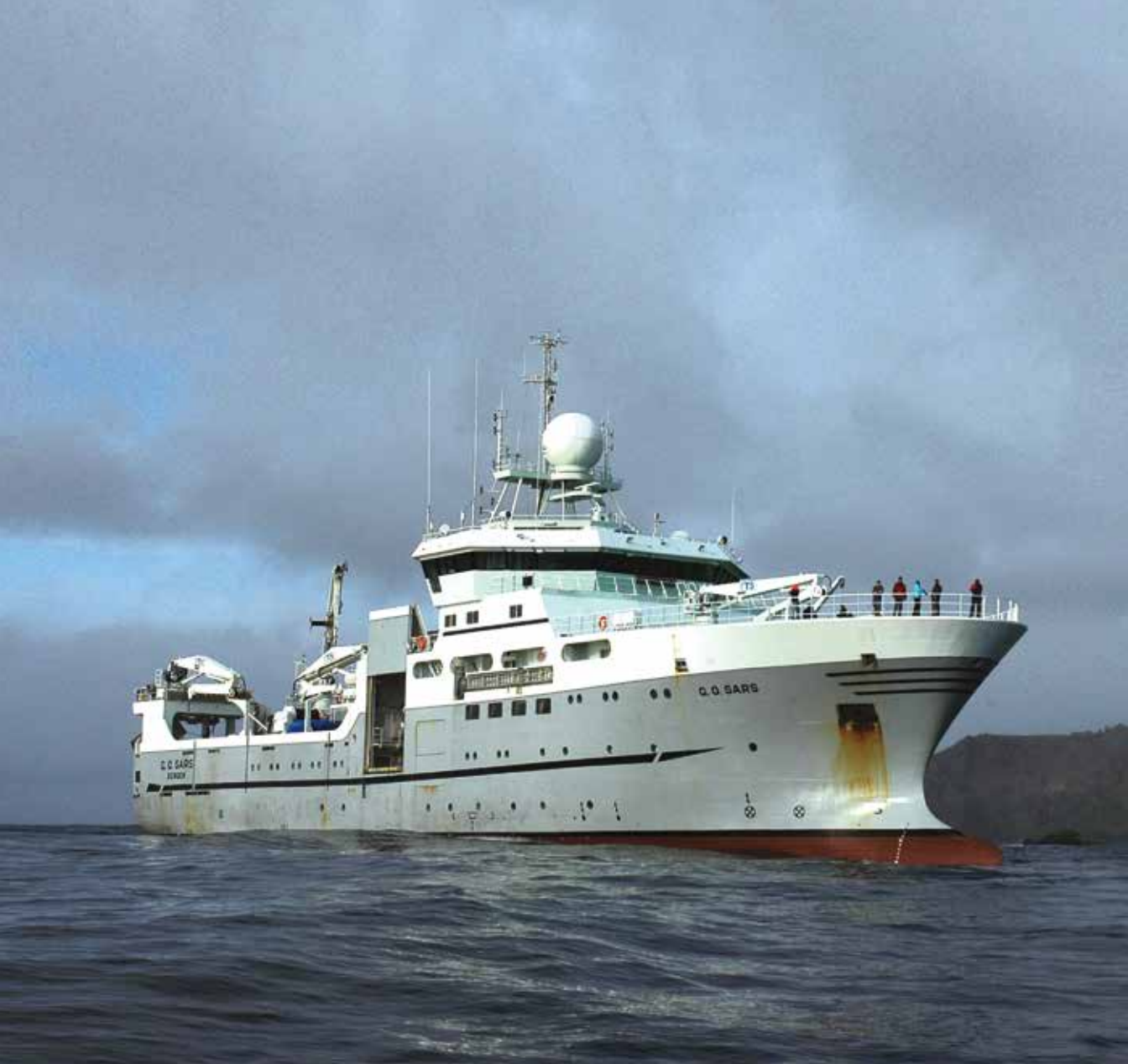
The Norwegian Institute of Marine Research's G.O. Sars is built to be super-quiet so as to have minimum impact on the sea and creatures being studied.
