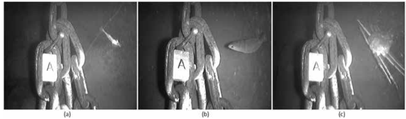
Figure 7: Images from an underwater video camera attached to the fishing line of the experimental-9 drop chain footgear trawl. Images show shrimp (a), turbot (b), and snow crab (c) in response to the approaching drop chain footgear.
