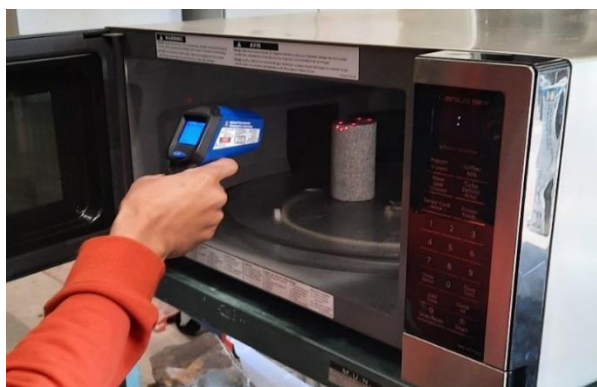
FIGURE 10: RECORDING TEMPERATURE OF A GRANITE SAMPLE BY USING AN INFRARED GUN.
