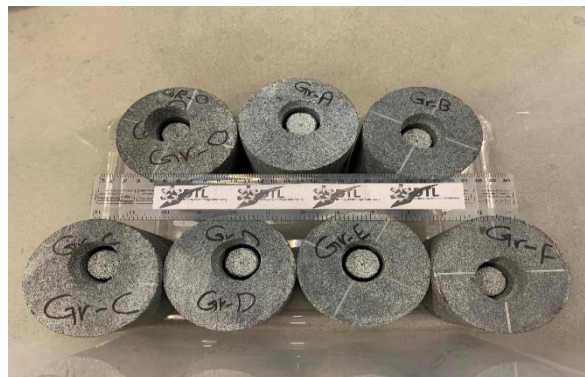
FIGURE 7: GRANITE SAMPLE AFTER DOT TEST ON SDS.
