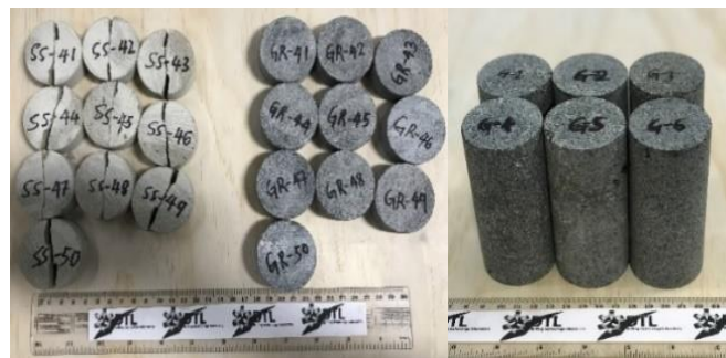
FIGURE 4: LEFT AND MIDDLE: UNHEATED-IT SAMPLES AND RIGHT: HEATED SAMPLES FOR ULTRASONIC WAVE TEST.
