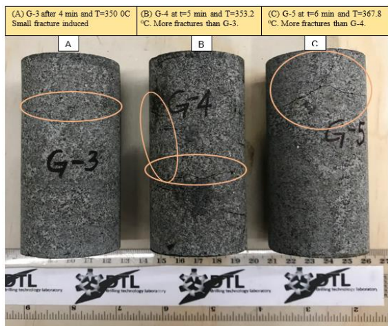
FIGURE 12: FRACTURES INDUCED ON 4IN- GR SAMPLE AFTER THE EFFECT OF RE-HEATED.
