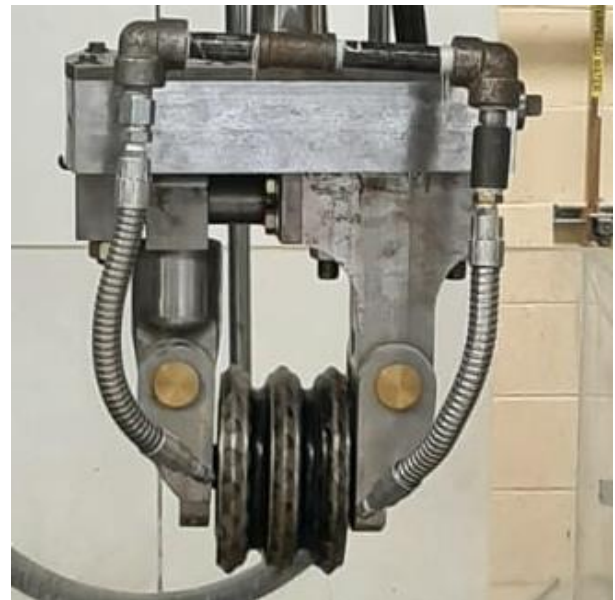
FIGURE 4: INSTALLED HIGH-PRESSURE SPRAY NOZZLE
