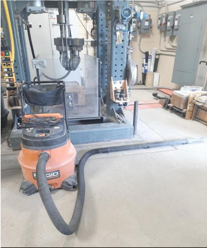
FIGURE 5: A 16US GALLON 6.5HP VACUUM CLEANER FOR CUTTINGS EVACUATION
