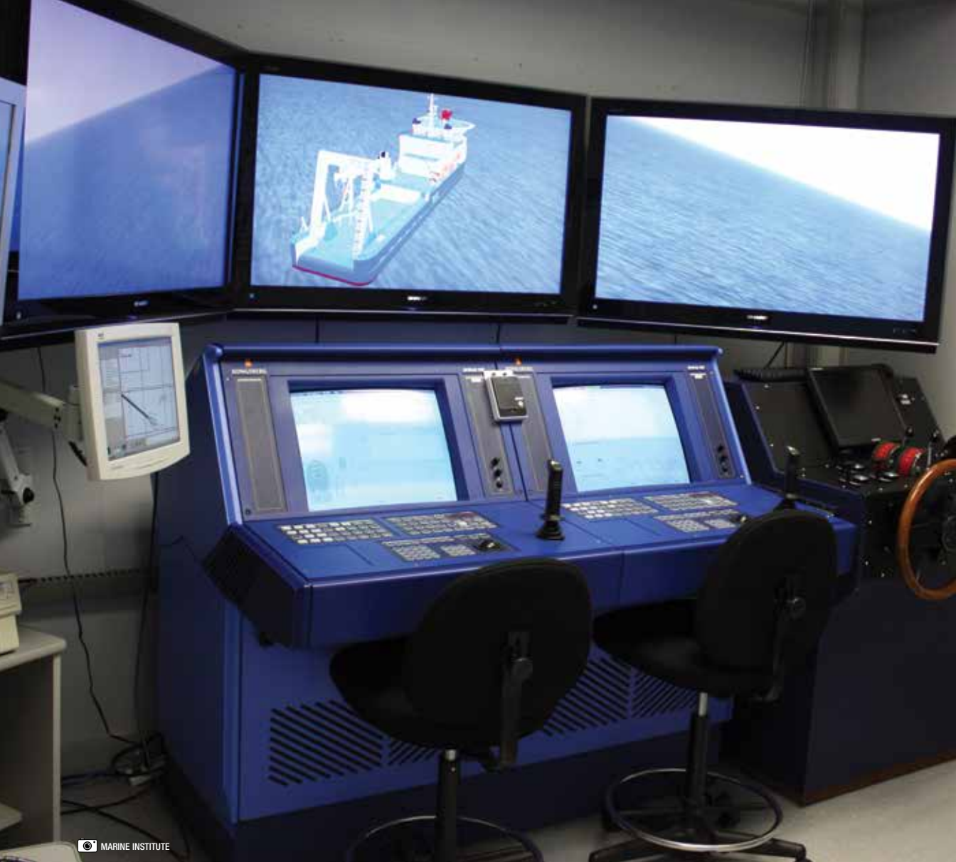
Figure 3: Both the SDP (left) and KPOS (right) Dynamic Positioning simulators are used to replicate precision manoeuvring systems.
