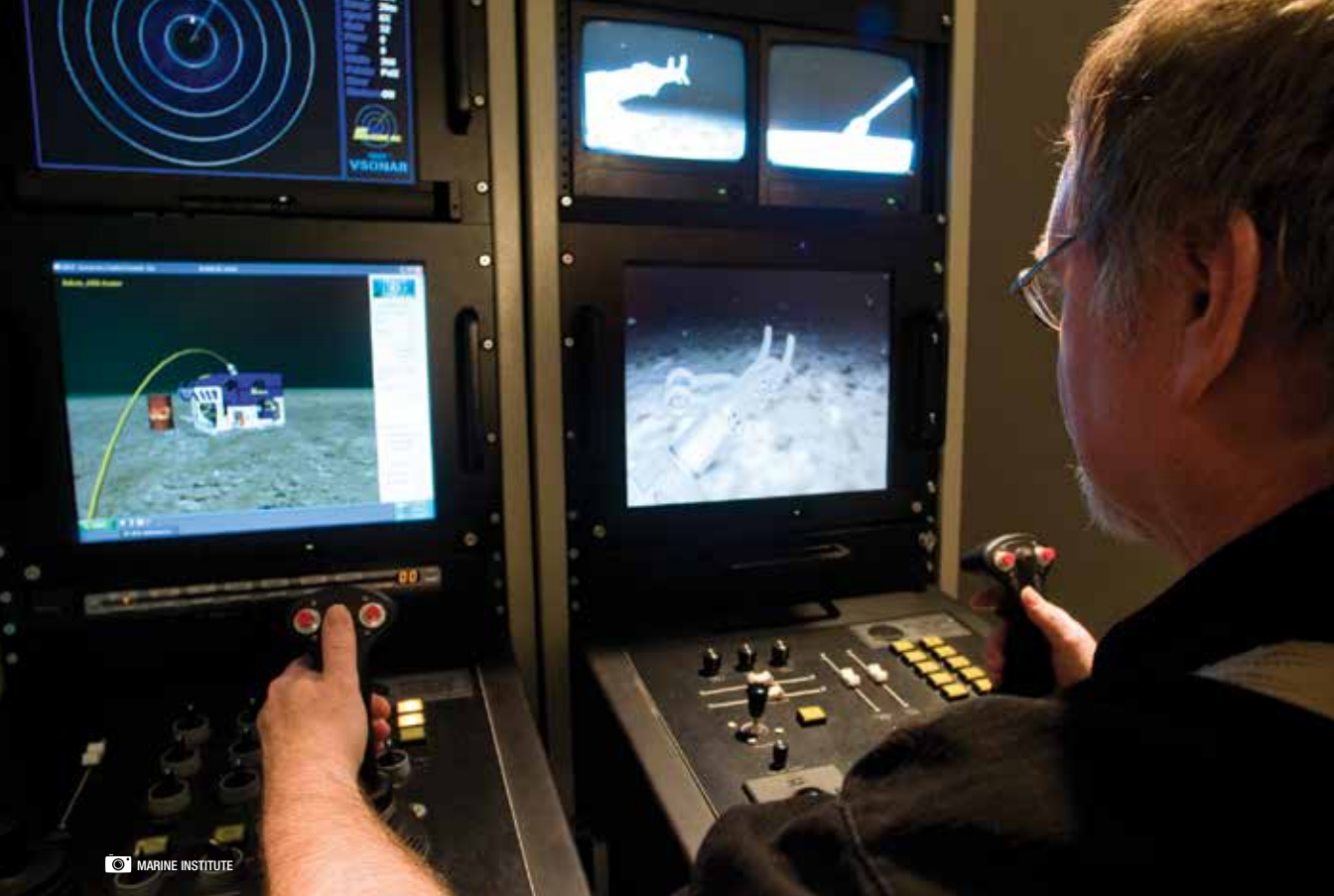
Figure 6: The Remotely Operated Vehicle simulator replicates the operations of offshore and military workclass vehicles.
