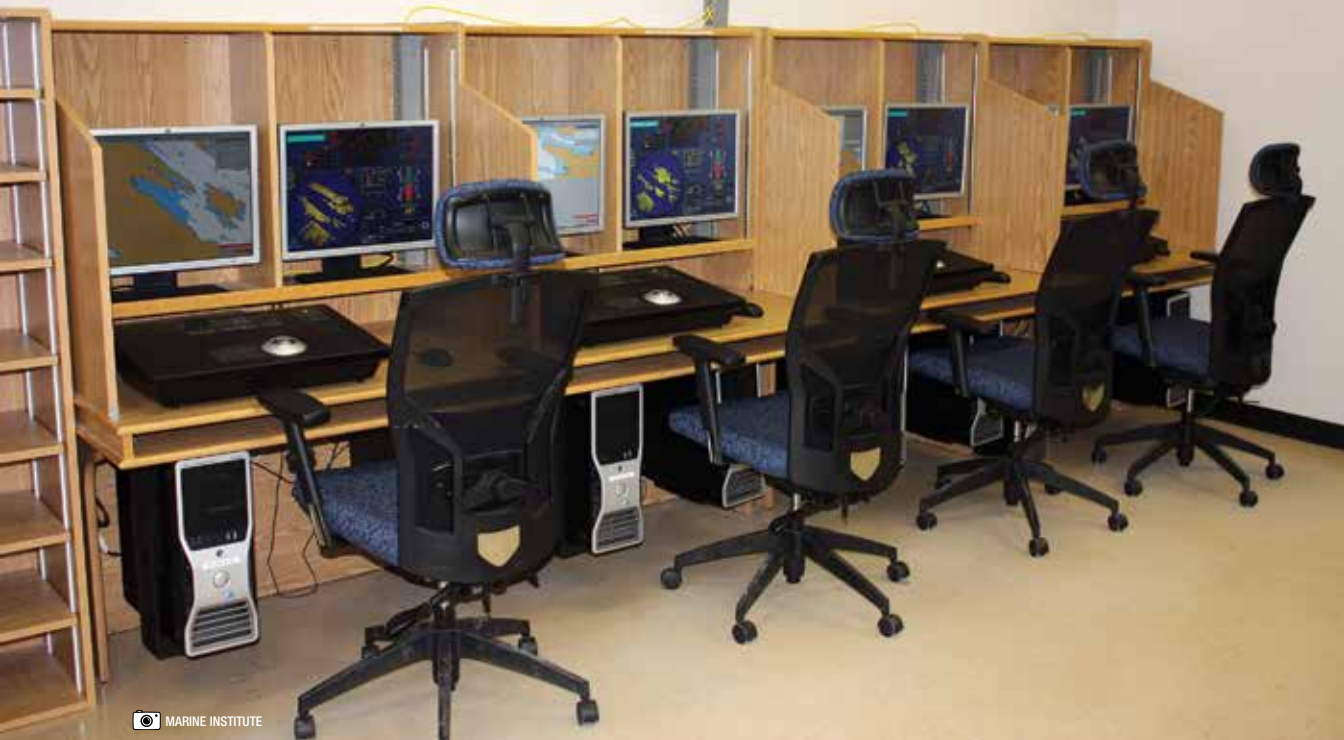
Figure 4: The Electronic Charting Display and Information System simulator displays information from system electronic navigational charts with positional information from navigation sensors to assist the mariner in route planning and monitoring.
