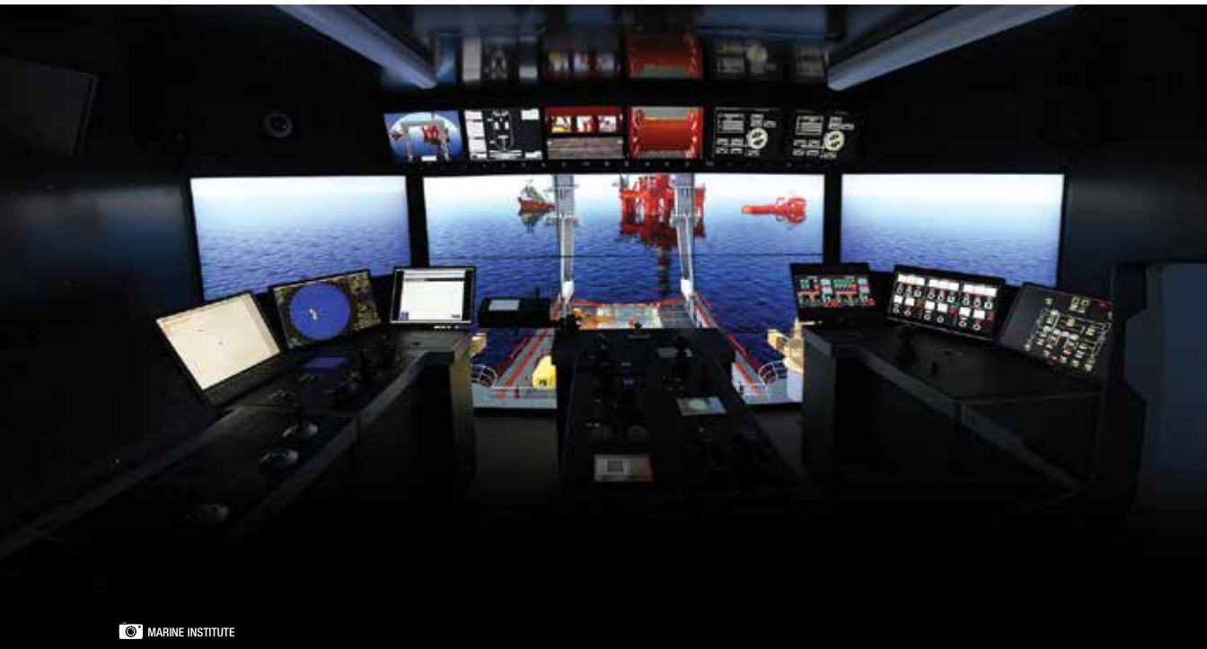
Figure 5: The Offshore Operations simulator is used to train personnel in positioning and mooring of offshore structures, deep water anchor handling, supply operations alongside platforms, iceberg management, and subsea operations.
