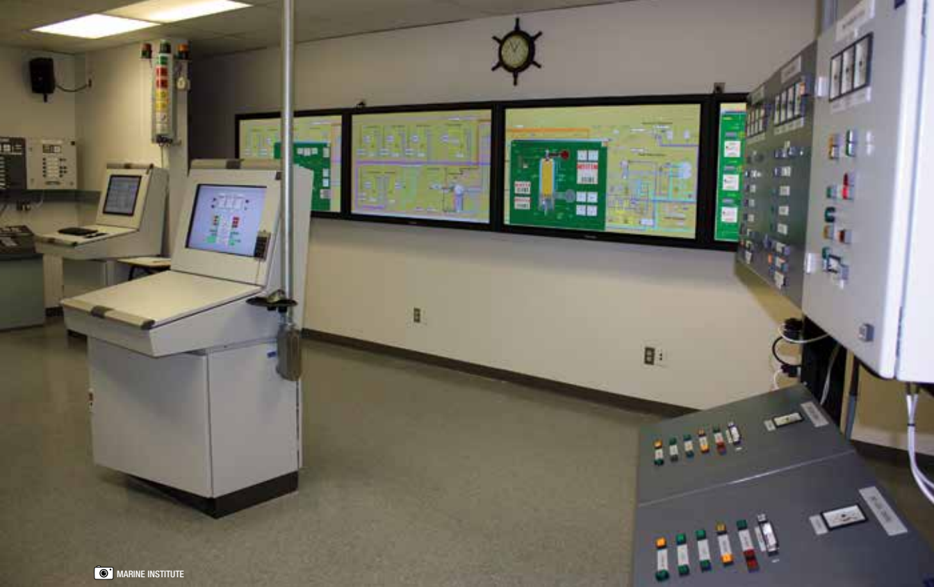
Figure 1: The Engine Room simulator with system display panels, switchboards, control room, and instructor station along with simulated slow and medium speed main engines.
