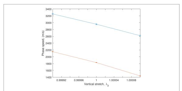
**Figure 2.** Calculation of phase speed variation for probe waves (P-wave (blue) and S-wave (red)) when perturbed by both a dynamic (sinusoidal) S-wave pump and a static pre-deformation  $\lambda$ , using the L-L model.
