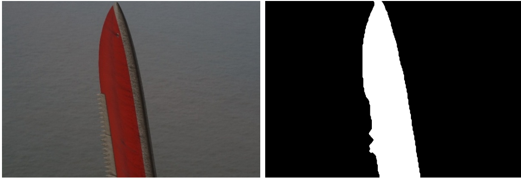
Figure 4.1: Sample image from Blade30 dataset showing the WTB and the respective segmentation mask
