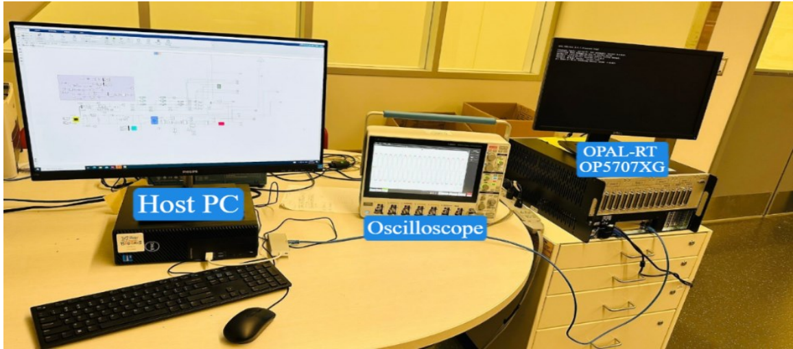
Figure 3. 28 OPAL-RT hardware setup.
