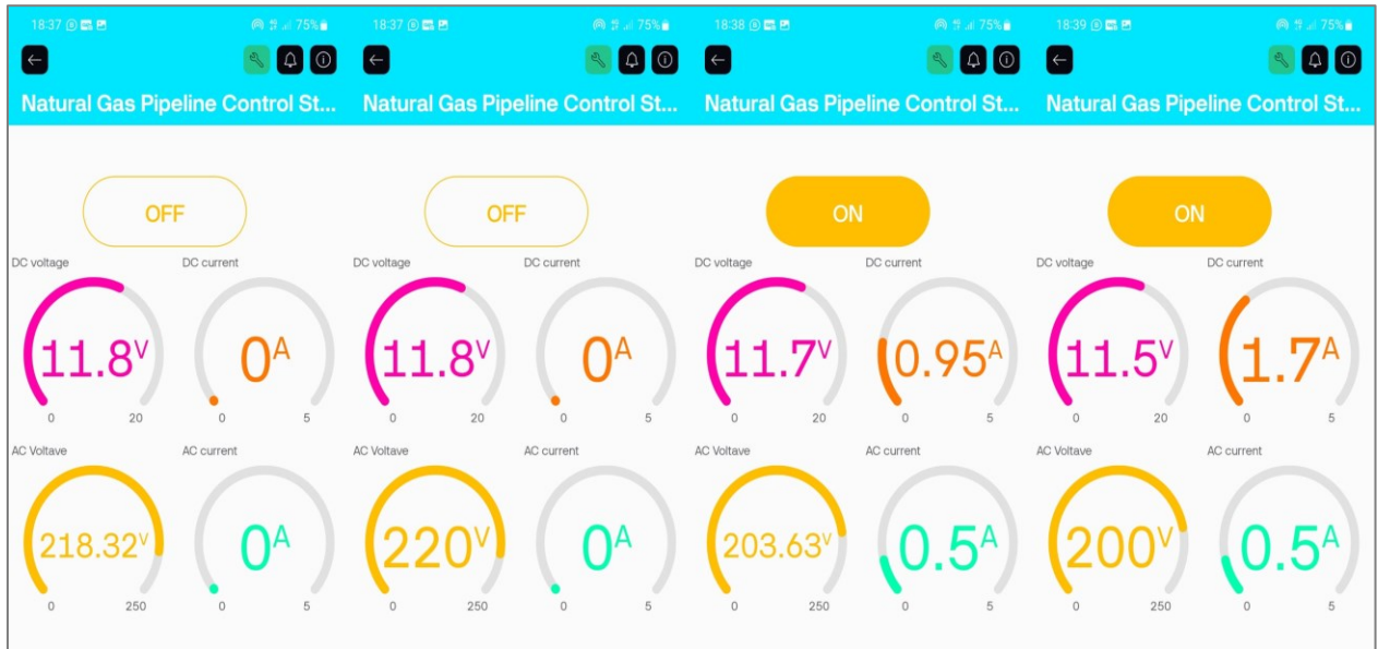
Figure 5.10. Display of FID parameters on Blynk mobile app using GSM SIM800L module with load OFF and ON.
