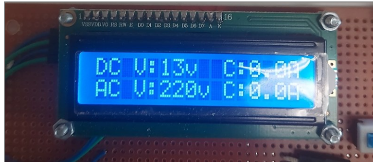
Figure 5.12. FID voltage and current display on the LCD when the load is off.
