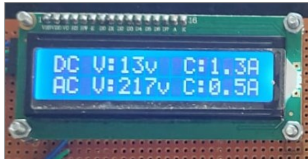
Figure 5.13. FID voltage and current display on the LCD.
