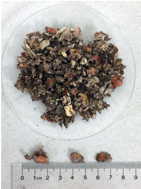
Figure 5: Air dried crab byproduct (L) before milling (13 mm particle size) and (R) after milling (1-2 mm).
