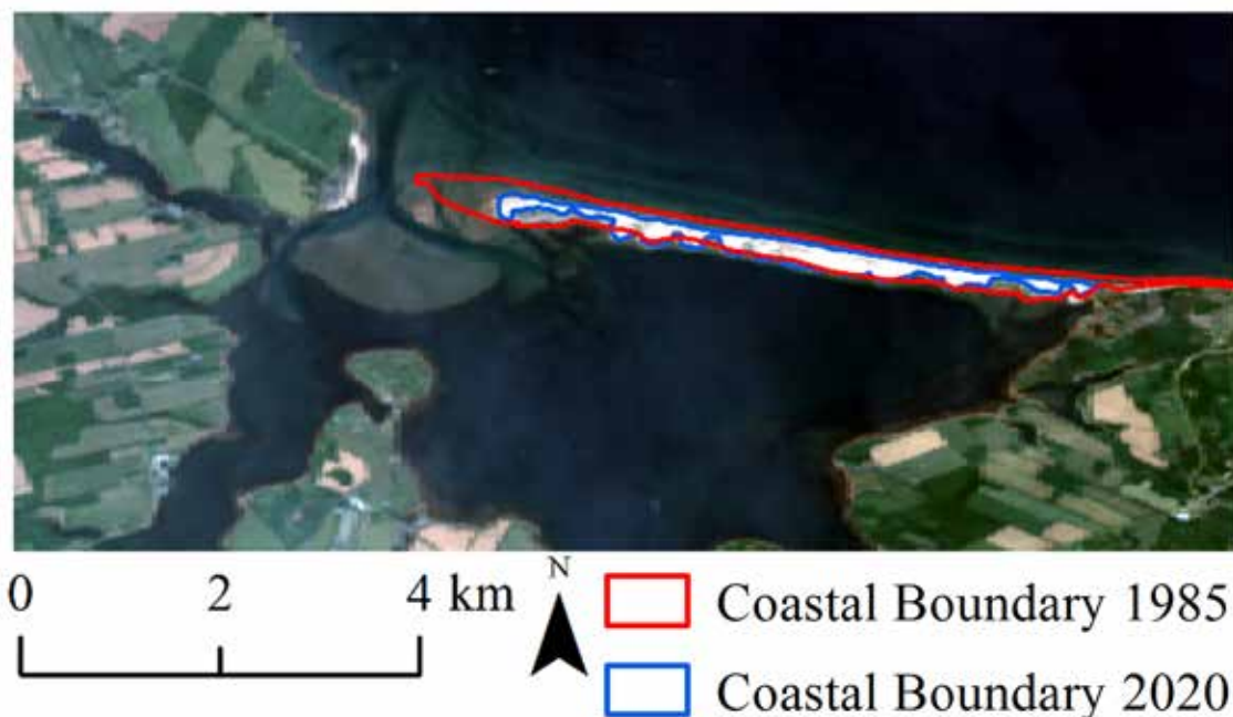
Figure 4: The boundary of coastal sand areas that was extracted based on the maps from Landsat imagery in 1985 and 2020.
