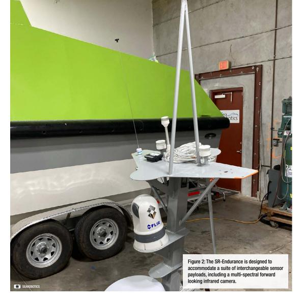
who designed the autopilot for the Mayflower autonomous ship, the ASV will change its route and behaviour to obey collision regulations and avoid collisions, while still attempting to accomplish its mission. Also on board are six cameras, including one multi-spectral forward looking infrared camera, providing a 360° view of the vehicle's surroundings (Figure 2).
