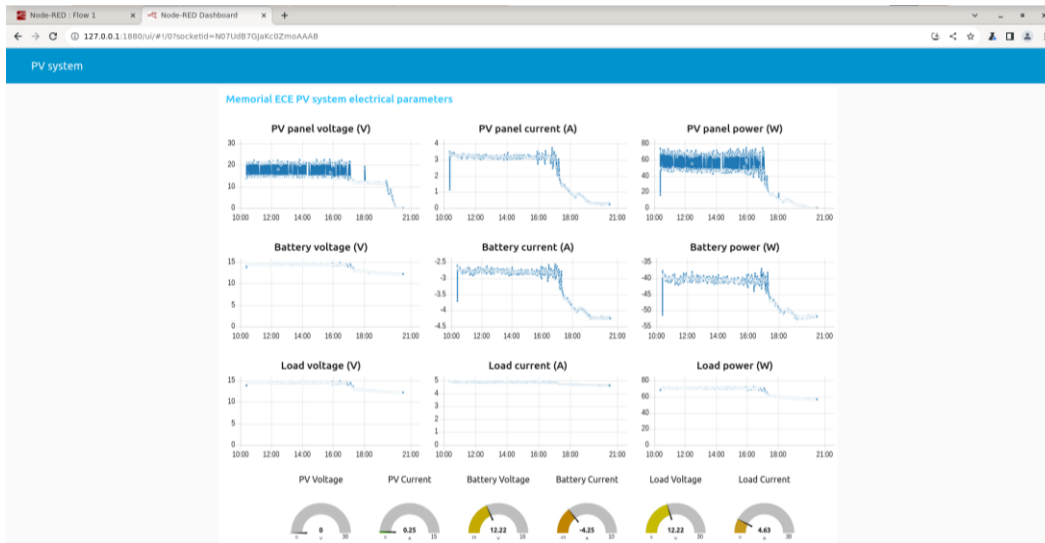
Figure 4-12 Node-RED dashboards showing the monitored values of the PV system.
