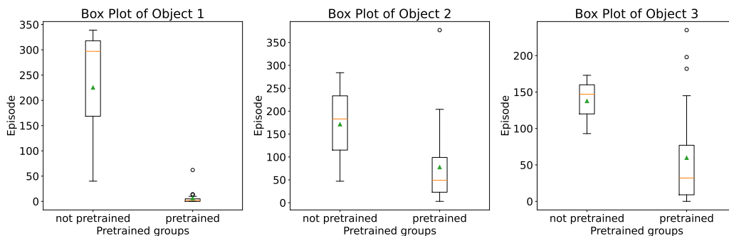
Figure 4.6: This figure shows a comparison between box plots of the number of episodes taken for a successful extraction with any form of pretraining and no pretraining for each object.
