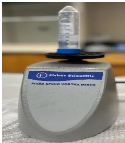
Figure 20. Vortex mixer: a laboratory instrument used to mix liquid samples through rapid rotational movement.
