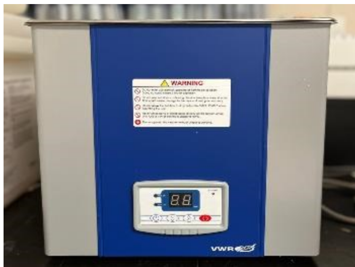
Figure 19. Suspensions are sonicated by using an ultrasonic cleaner.
