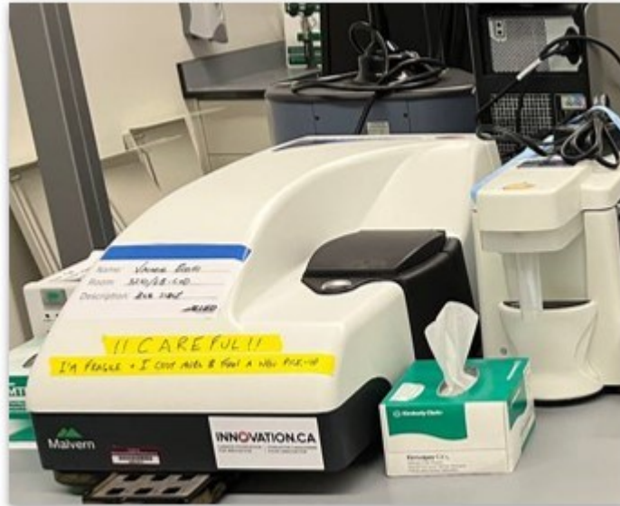
Figure 15. Zeta sizer, a device for analyzing particle suspensions by measuring light scattering, particle size, and zeta potential (ZP).
