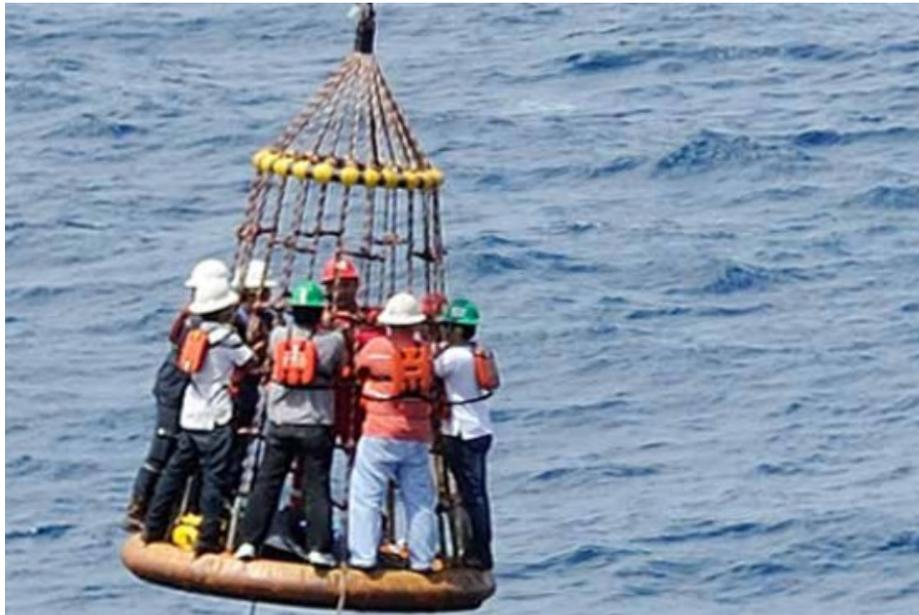
**Figure 1-2: Collapsible Net Crew Transfer [20]**
