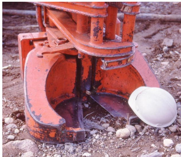
Figure 16 Shear head on the prototype Timberjack harvester-processor. The pressure exerted by these felling heads tended to splinter tree trunks. (Malcolm Squires Photo).
