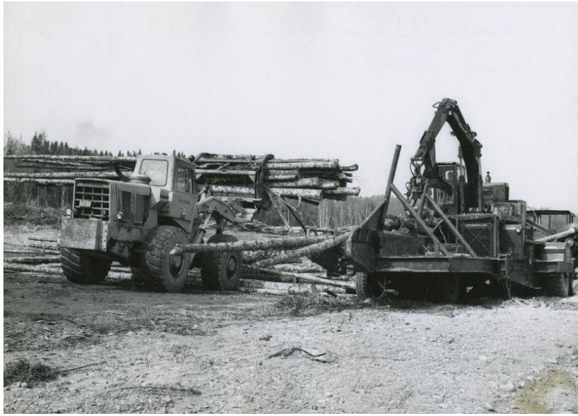
Figure 13 Slasher and loader 1971. Note the size of the slasher compared to the front-end loader, early slashers were mobile in that they could be moved, in practice moving them was difficult. (GFWHS)
