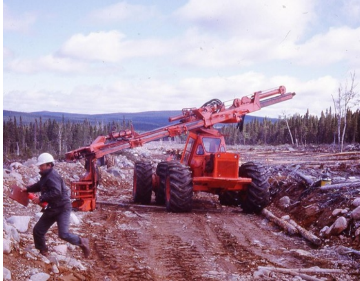
Figure 14 Prototype Timberjack feller-delimber, Pamehac, July 1971 (Malcolm Squires)
