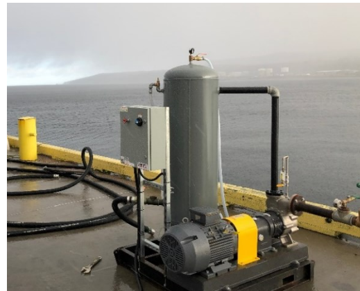
Fig. 4.2: The Nikuni KTM65S2 bubble generator setup at the Holyrood wharf
