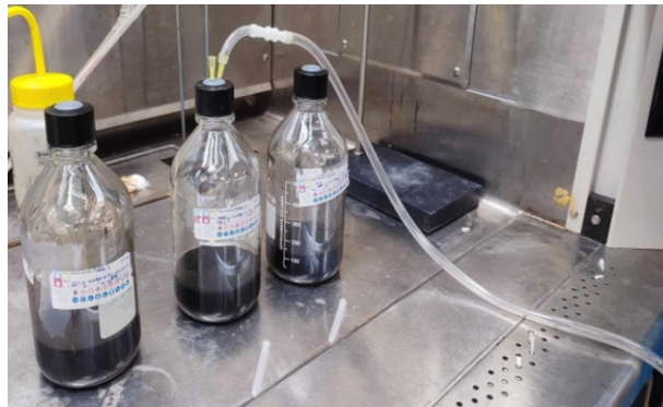
Figure 5- 1. Nitrogen gas is purged through the culture and substrate, ensuring the maintenance of anaerobic conditions in each digester.
