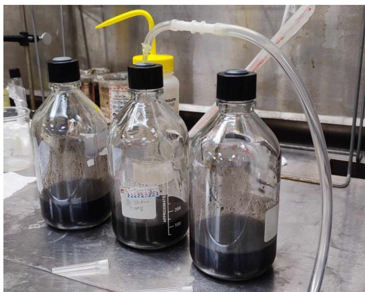
Figure 6- 1. Nitrogen gas is flushed in each digester to sustain an anaerobic environment.
