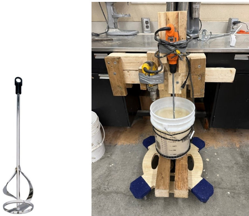
Figure 5-1: Hand drill mixing blade and experimental setup
