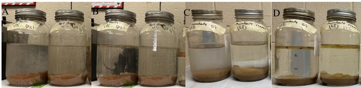
Figure 5-6: Water settlement test for imaging fluid mixed at 3000 rpm and low temperature in 5 and 24°C a) API barite (oven-heated) after 1 hr b) after 7 days c) Microbarite after 1 hr d) after 24 hrs
