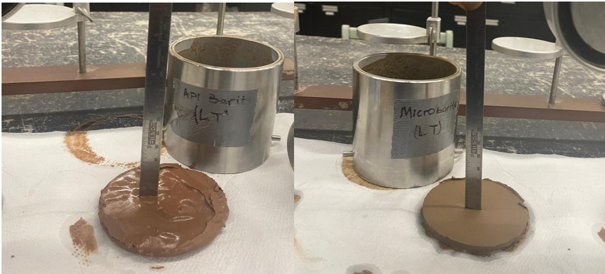
Figure 5-11: Filtration test mud cake for imaging fluid produced using 3000 rpm (+ oven heated for API barite) mixed at low temperature
