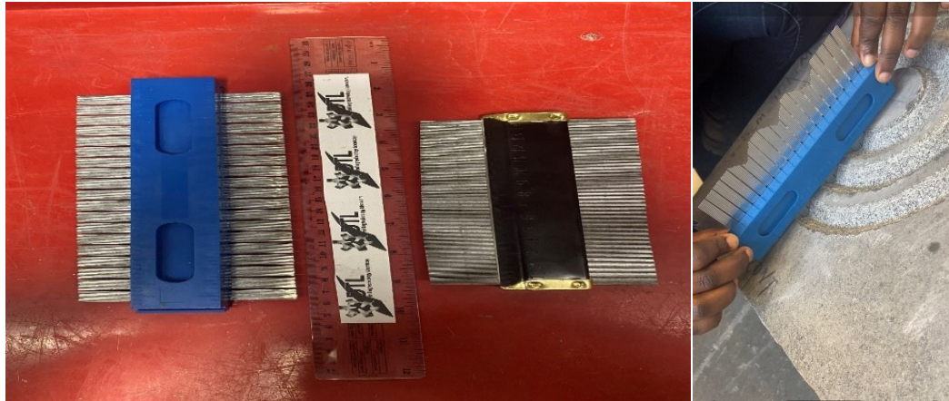
Figure 4-6: Contour gauge used for groove mapping
