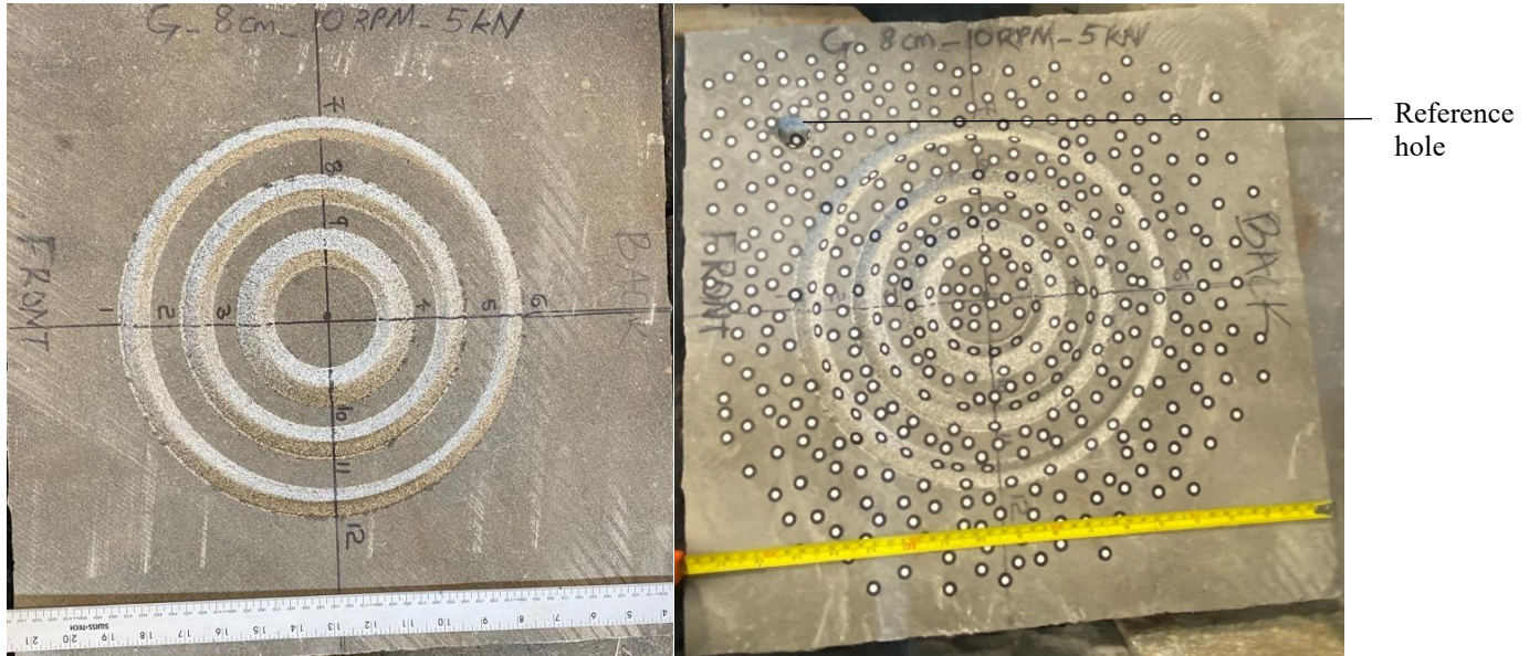
Figure 4-9: Rock specimen with markers and reference hole
