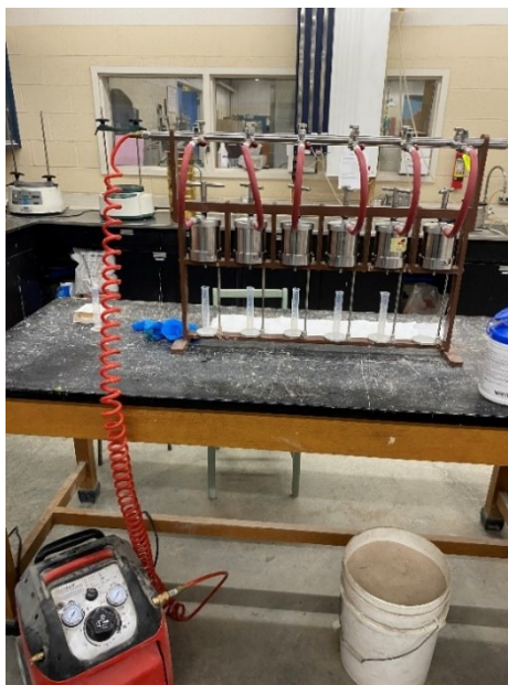
Figure 5-3: (A) OFITE 8-speed rotational viscometer (B) API fluid loss test kit
