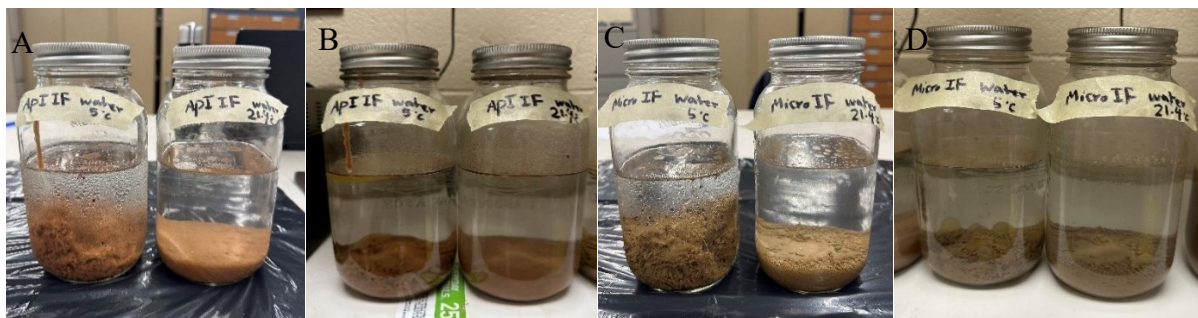
Figure 5-7: Water settlement test for imaging fluid mixed using the general protocol in 5 and 24°C a) API barite after 1 hr b) after 7 days c) Microbarite after 1 hr d) after 7 days
