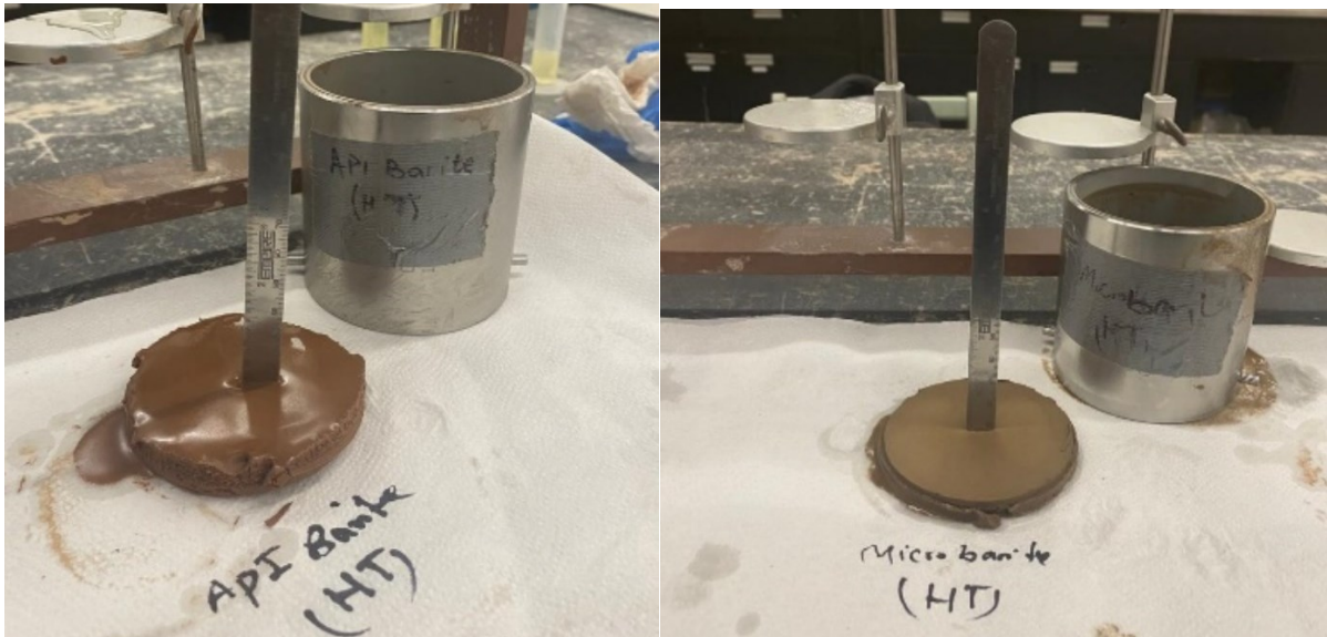
Figure 5-10: Filtration test mud cake for imaging fluid produced using 3000 rpm mixed at high temperature
