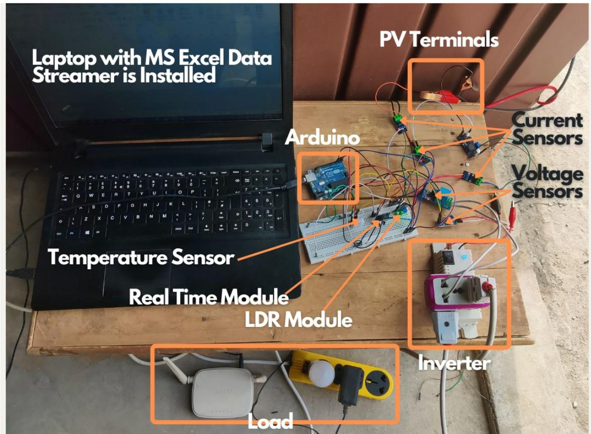
Figure 4.10 Experimental Setup
