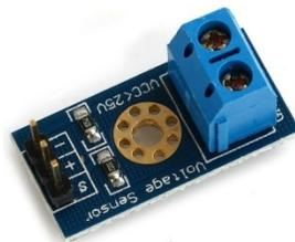
Figure 4.5 DC Voltage Sensor
