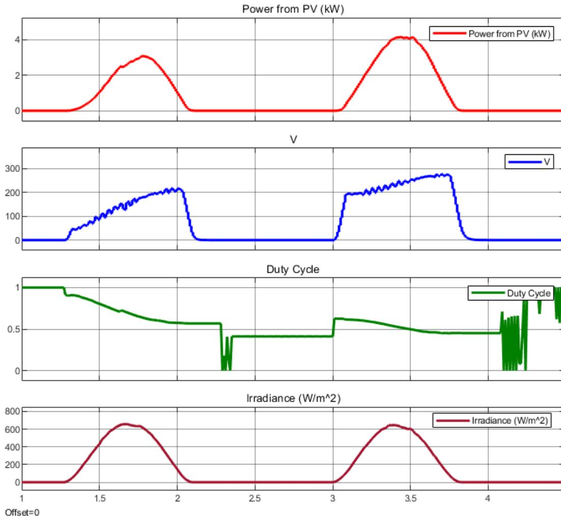
Figure 3.10 Realistic Irradiance to simulate day and night cycle
