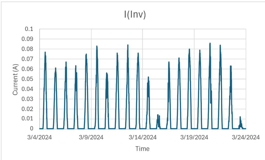
Figure 4.15 Inverter current measured using curent sensor.
