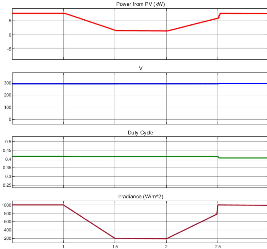
Figure 3.8 Varying Irradiance from 1000 W/m<sup>2</sup> to 200 W/m<sup>2</sup>
