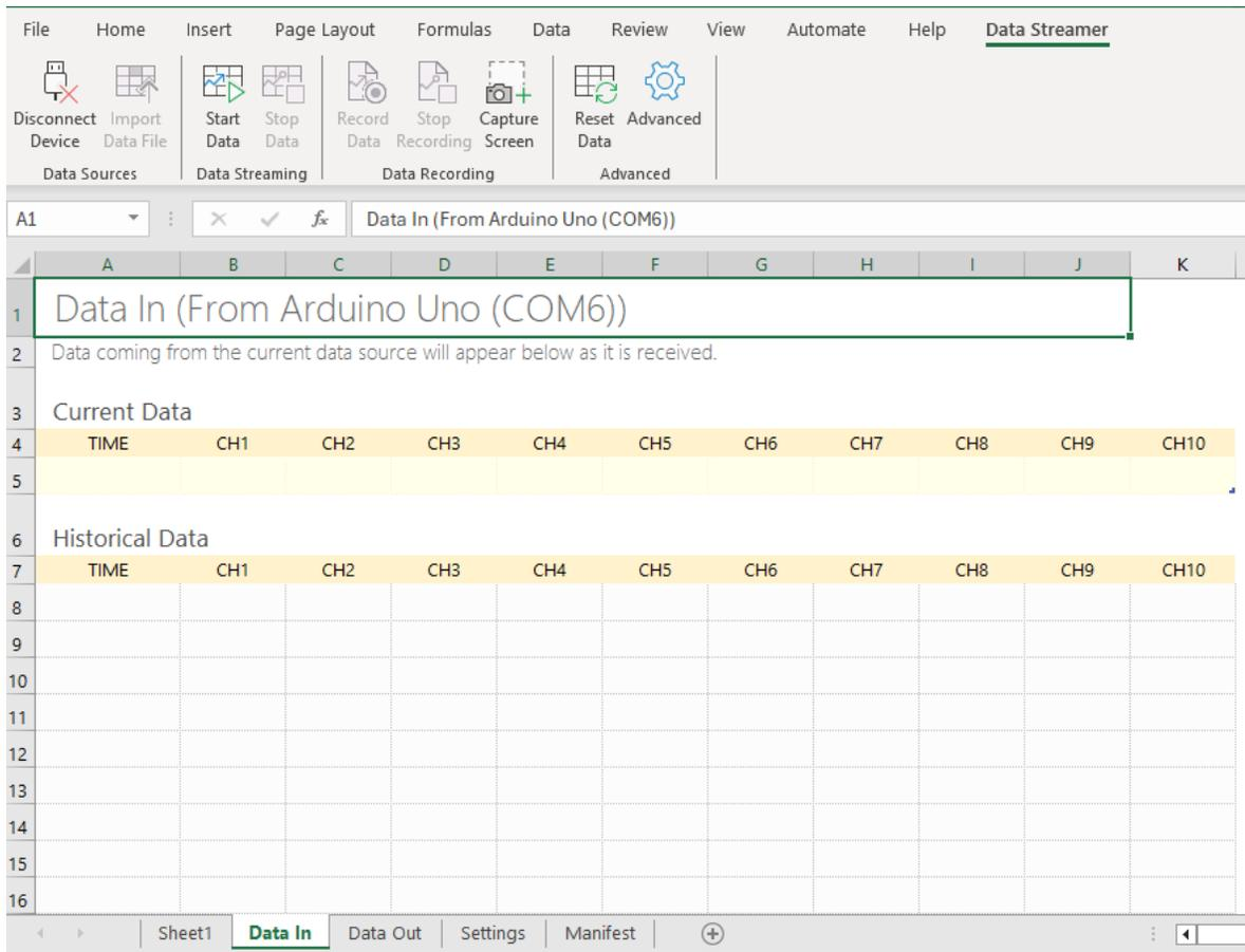
Figure 4.11 MS Excel Data Streamer Interface
