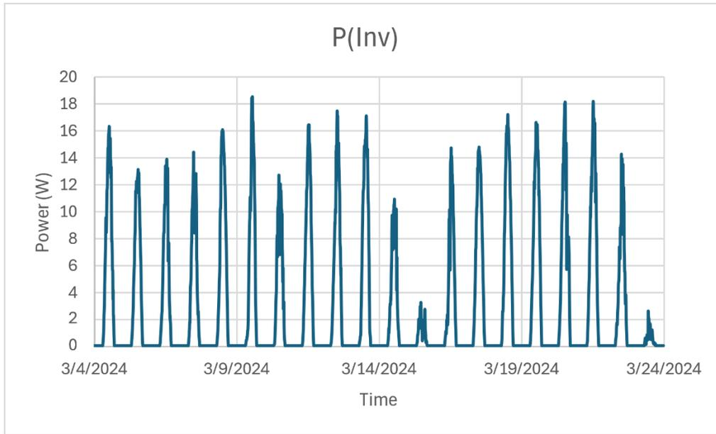
Figure 4.16 Output power calculated using Inverter voltage and inverter current.
