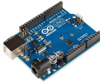
Figure 4.2 Arduino UNO utilized in this study.
