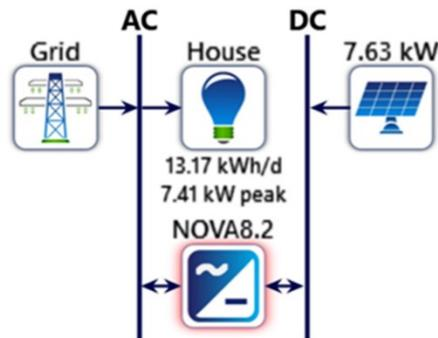
Figure 2.8 System Structure in Homer Pro
