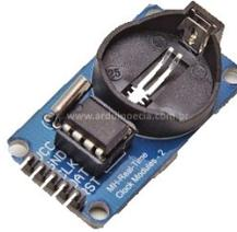
Figure 4.7 Real Time Clock Module for timestamping.
