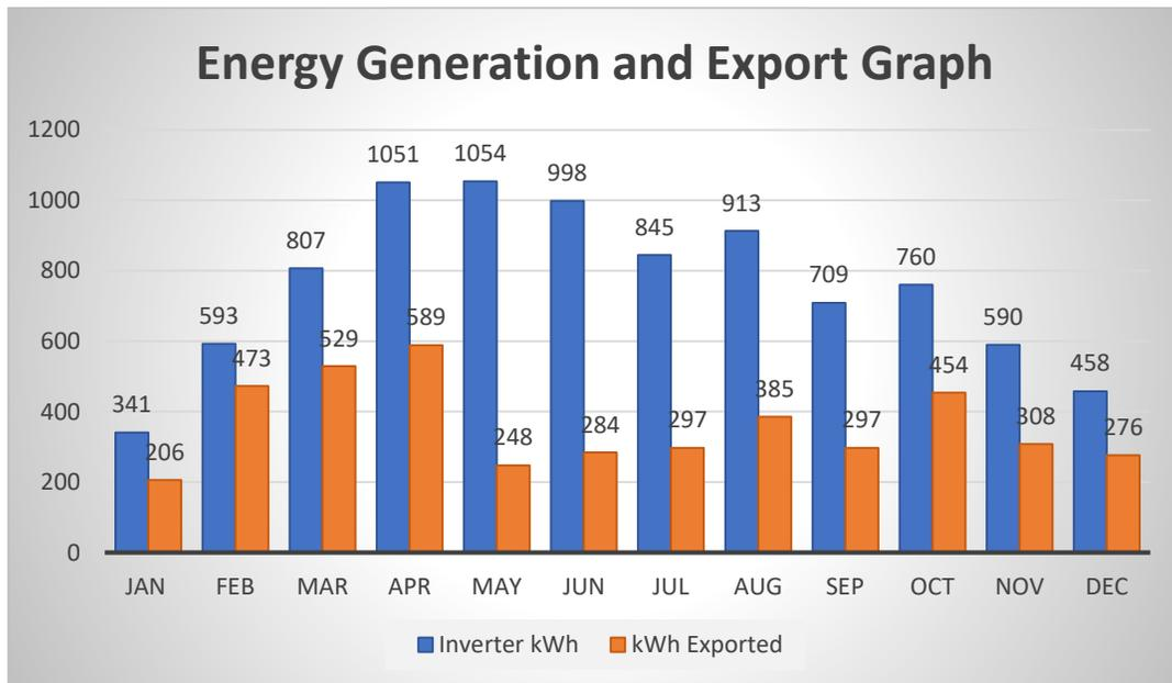
Figure 2.6 Monthly Energy Production Log of Inverter
