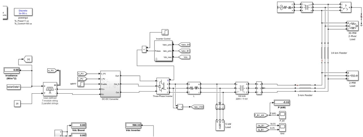
Figure 3.1 Overall structure of the installed system modelled in Simulink
