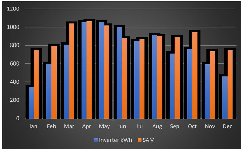
Figure 2.15. Comparison Chart of Inverter Output and SAM Results.
