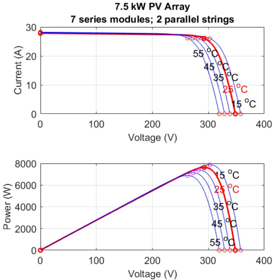
Figure 3.2 I-V and P-V Curves of the PV Array
