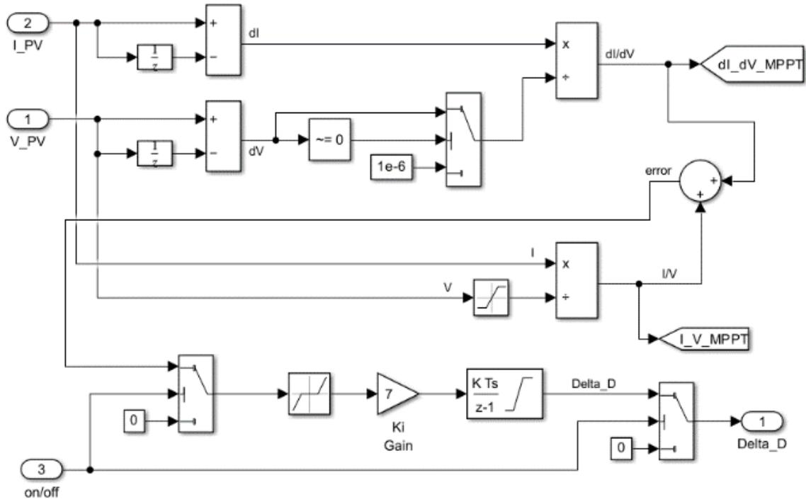
Figure 3.4 MPPT Controller for DC-DC Converter
