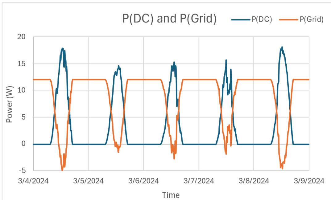
Figure 4.17 Power provided by PV and grid during day and night sessions for first 5 days.
