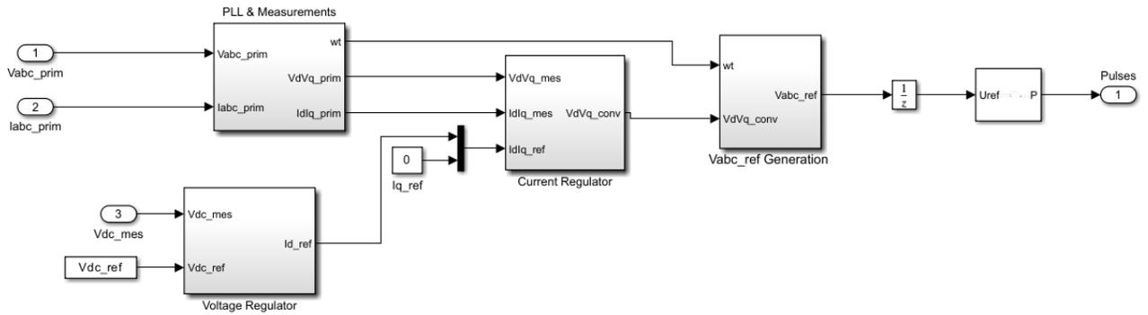
Figure 3.5 MPPT Controller for Three-Phase Inverter
