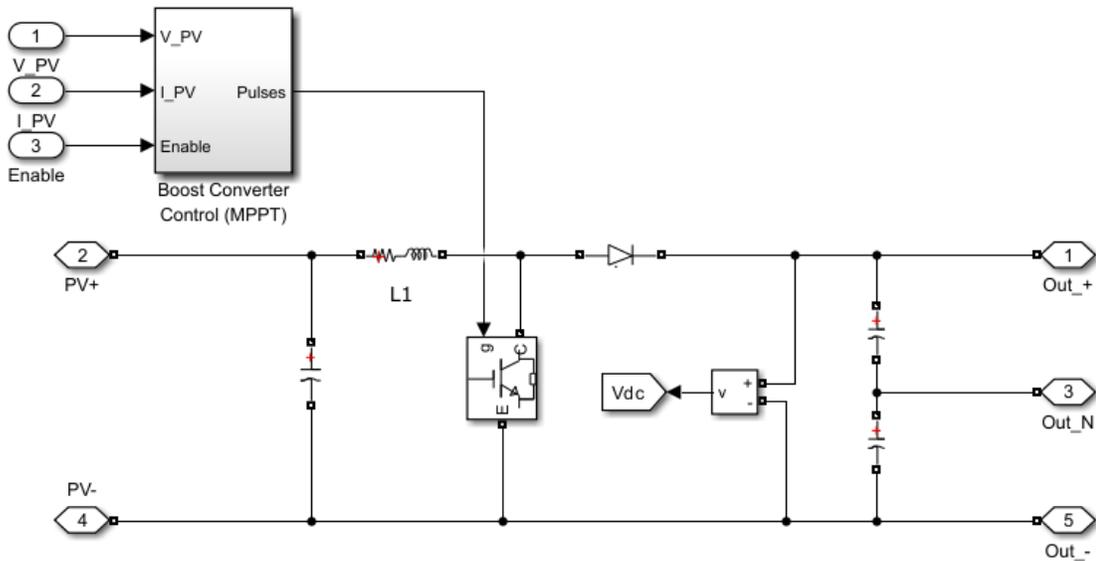
Figure 3.3 DC-DC Converter
