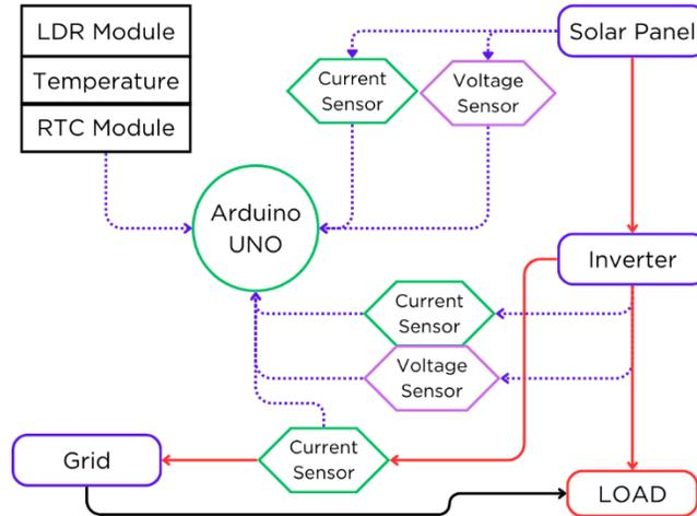
Figure 4.8 Overall block diagram of the proposed study. Here, the red and black lines illustrate the power flow while blue dotted lines shows the connection of sensors with Arduino.
