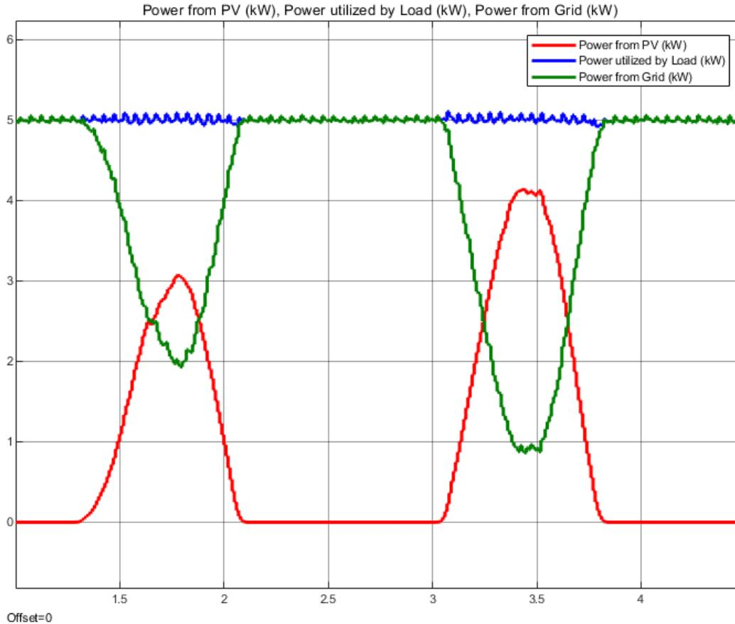
Figure 3.11 Power generation of PV and Grid along with Power utilized by the load during Day and Night scenario.
