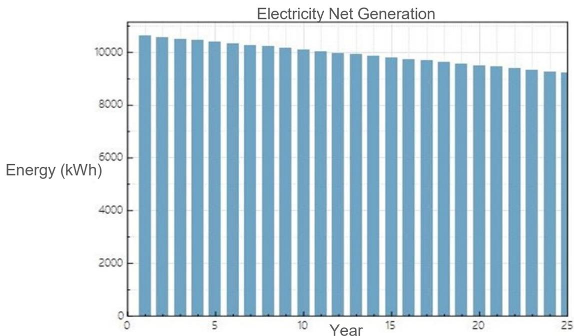
Figure 2.14 Projected Energy of the system for 25 years
