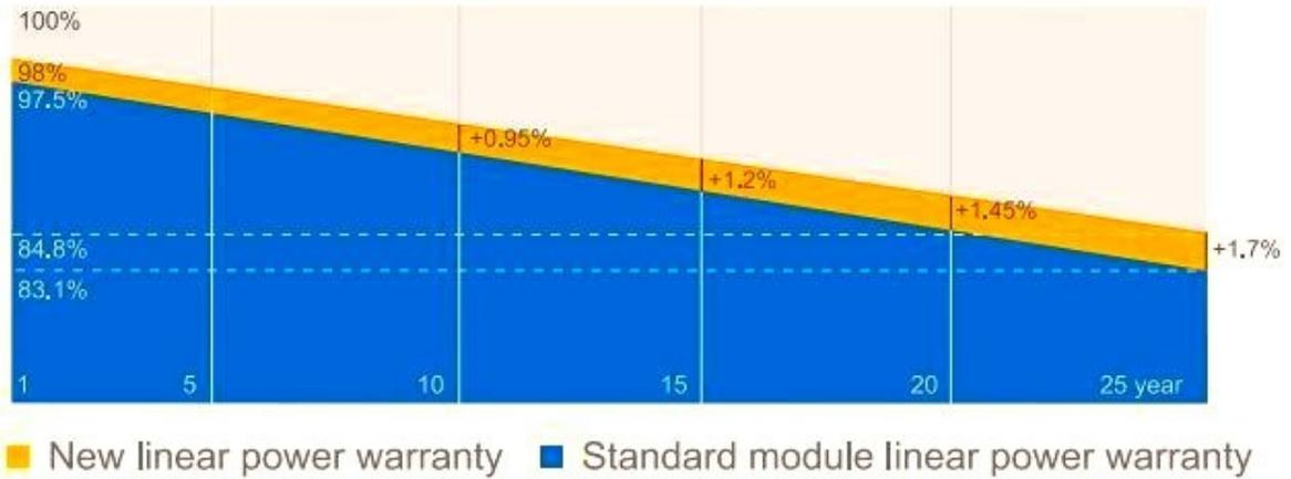
Figure 2.3 Projected efficiency of Solar Panel for 25 years [3].
