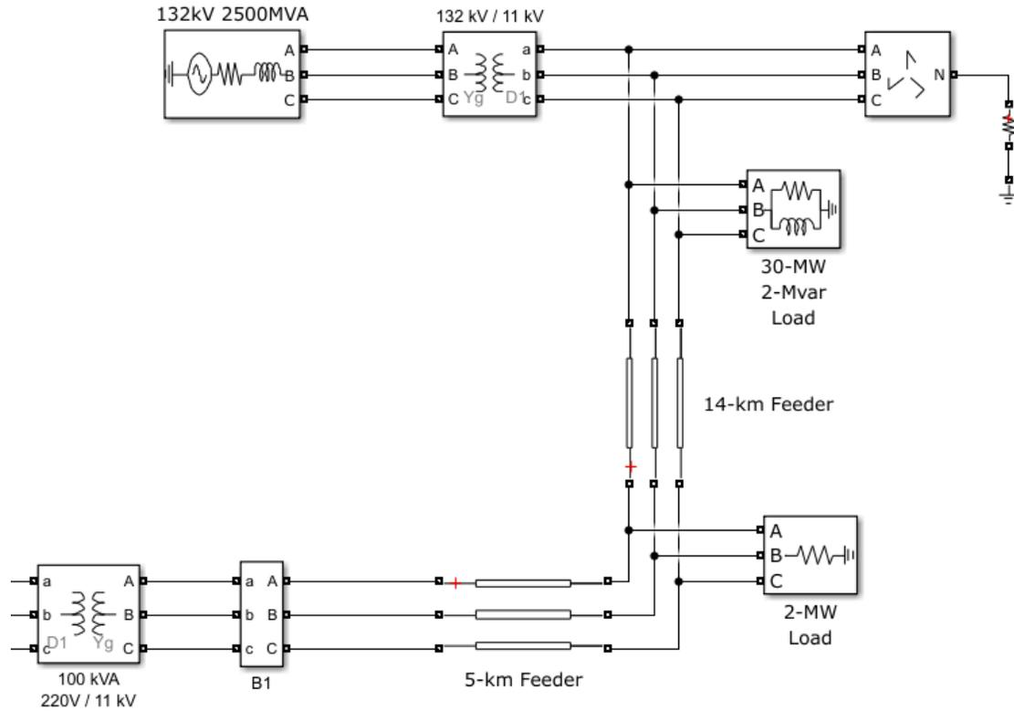
Figure 3.6 Three-Phase Grid modelled in Simulink
