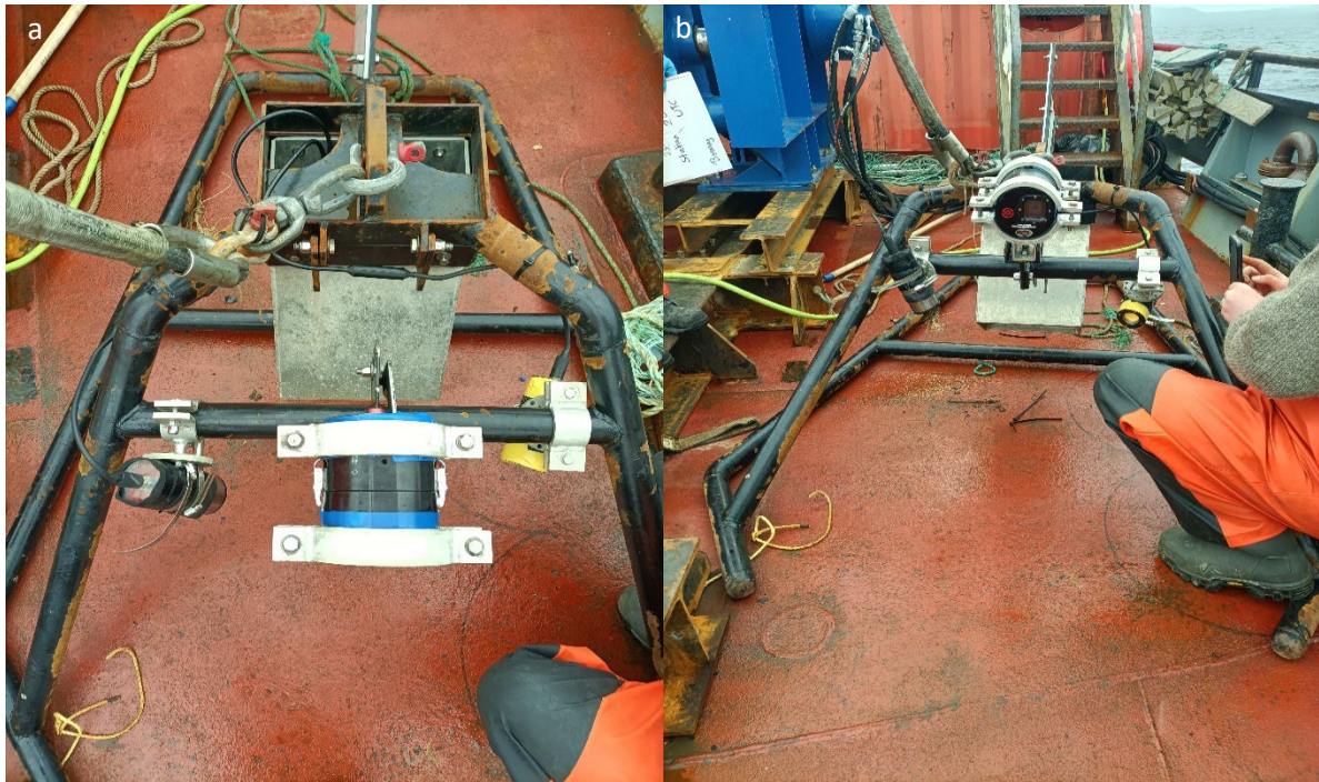
Figure 6: Bounce Camera configuration (a) for the down-facing camera and (b) with the forward-facing camera with additional Subsea lamp (left of the forward-facing camera) removed from the Drop Camera. Photos: E Broad.
