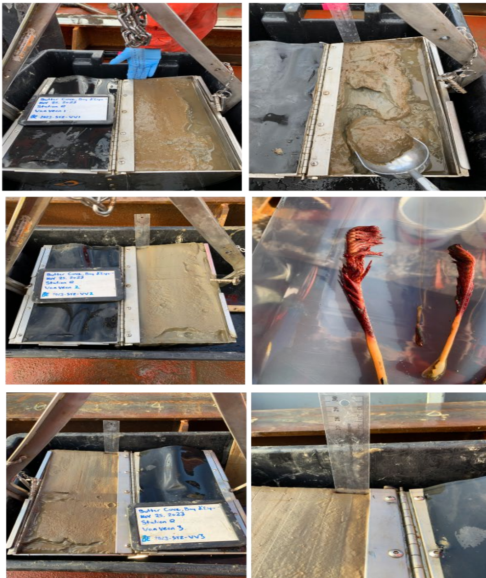
Figure 11: Three successful Van Veen grab replicates from Bay d’Espoir. Photo: V. Hayes.
