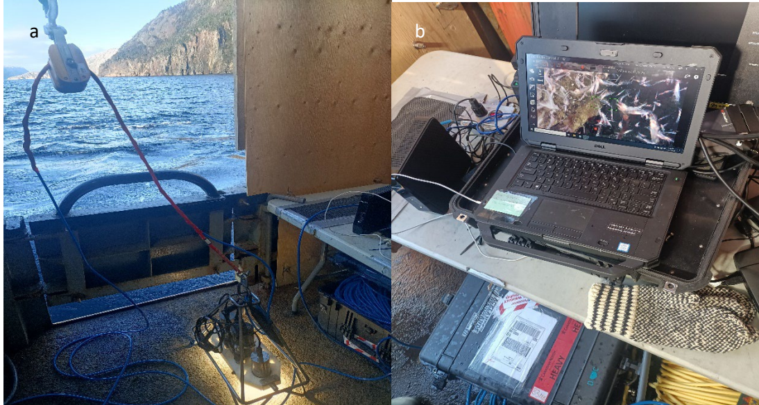
Figure 5: On-deck configuration for Drop Camera deployment (a) configuration for deployment/recovery (b) dry set up of the BCP unit, ethernet, and Sub-C software on dedicated field laptop. Photos: E Broad.
