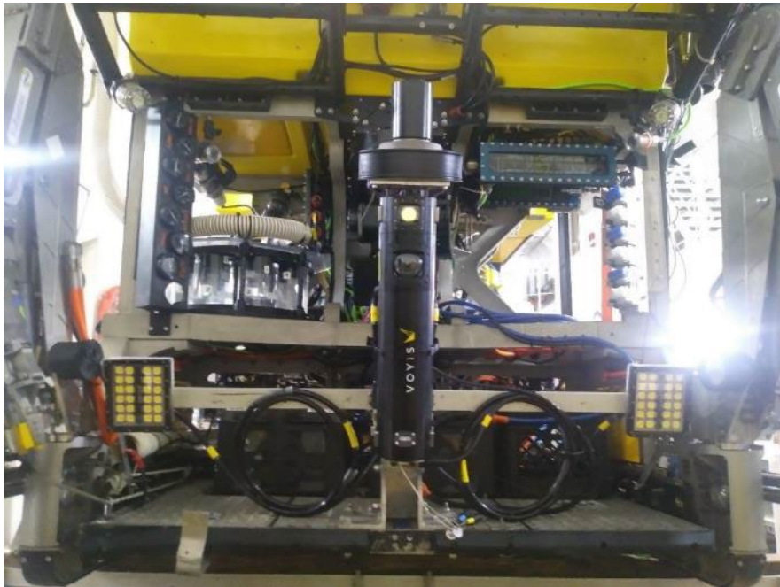
Figure 11: Mounting of Voyis laser for dive S0584 at 75 degree, with LED panel on either side and Norbit MBES mounted on top.
