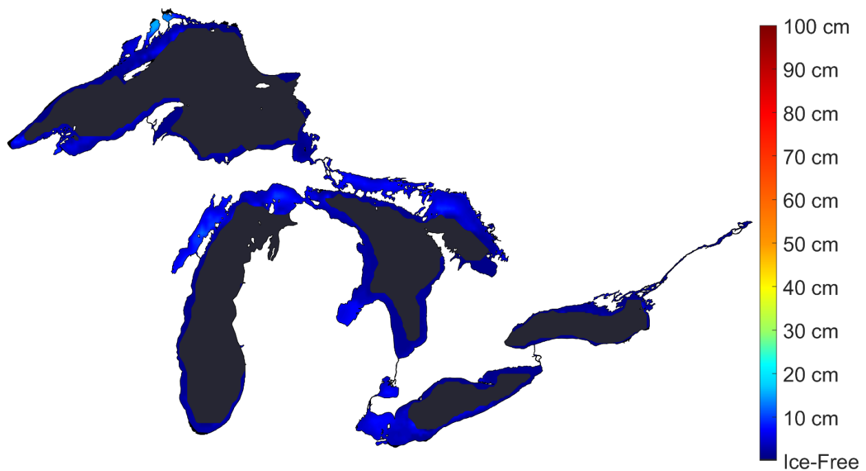
Figure 4-7: Spatial distribution of daily-averaged equivalent ice thickness throughout the Great Lakes for days with ice present during the month of December from 2009 to 2018.
