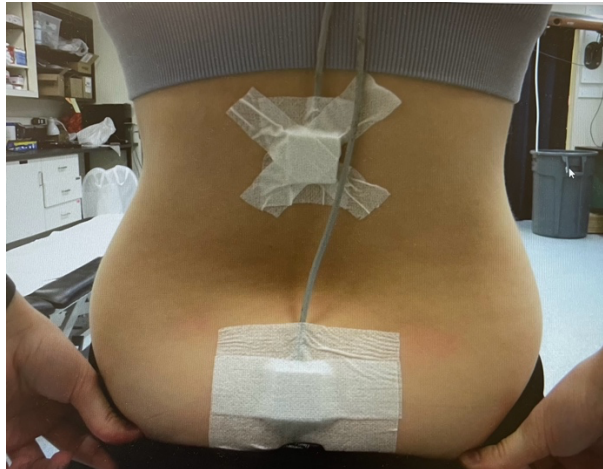
Figure 7: Accelerometer placement on L1 and S2 spinous processes.
