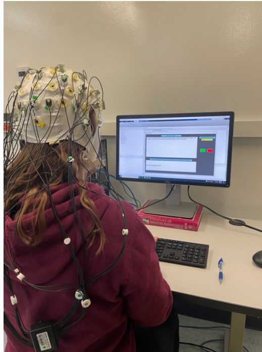
Figure 11: Participant seated at the ergonomic workstation instrumented with the EEG and accelerometers.
