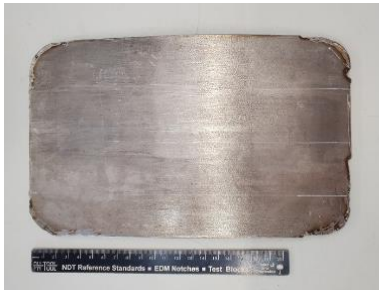
Figure 4 A section of a MIC damaged pressure vessel plate seen from the outside surface is used for the case study.
