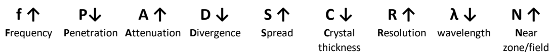
Figure 7 A mnemonic is used in NDT/NDE training to highlight the relationship of variables in UT.
