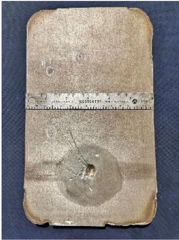
Figure 5 Visual examination of the internal surface of the test plate. Pits 1 and 2 are highlighted pit 3 is the large pit in the bottom centre of the plate.
