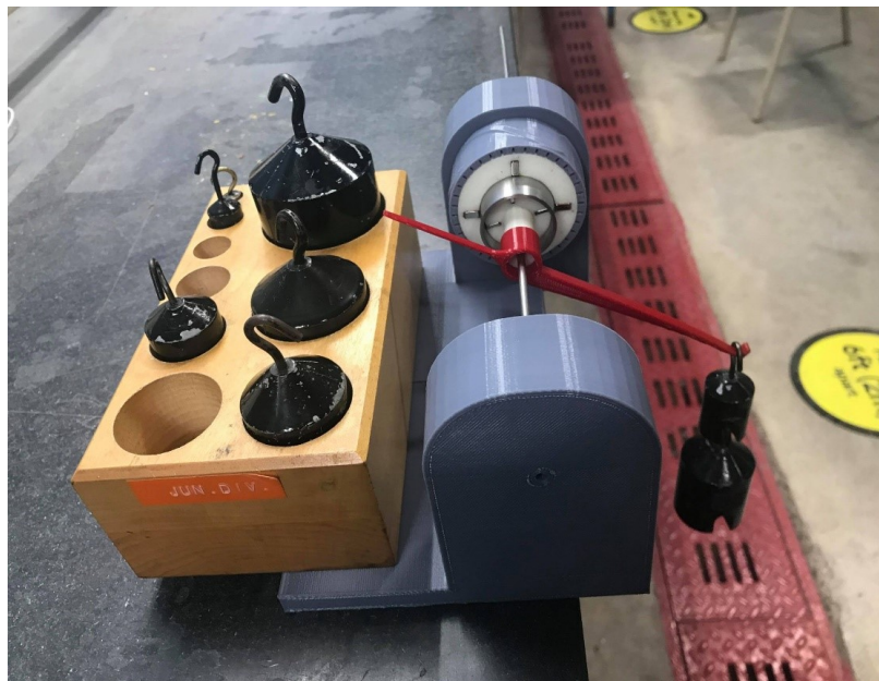
Figure A.3 Slip and Torque Test Set up
