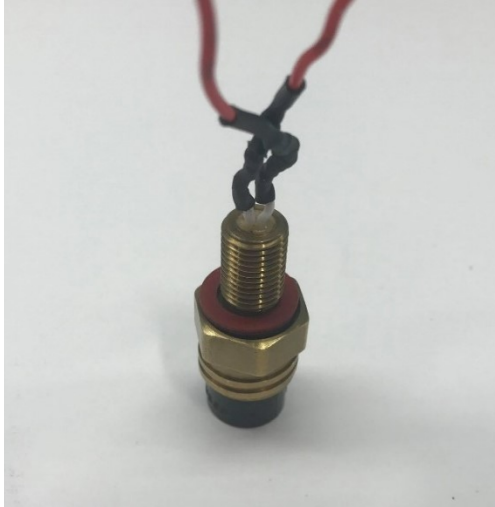
Figure 3.9 Waterproof Subcon Connection
