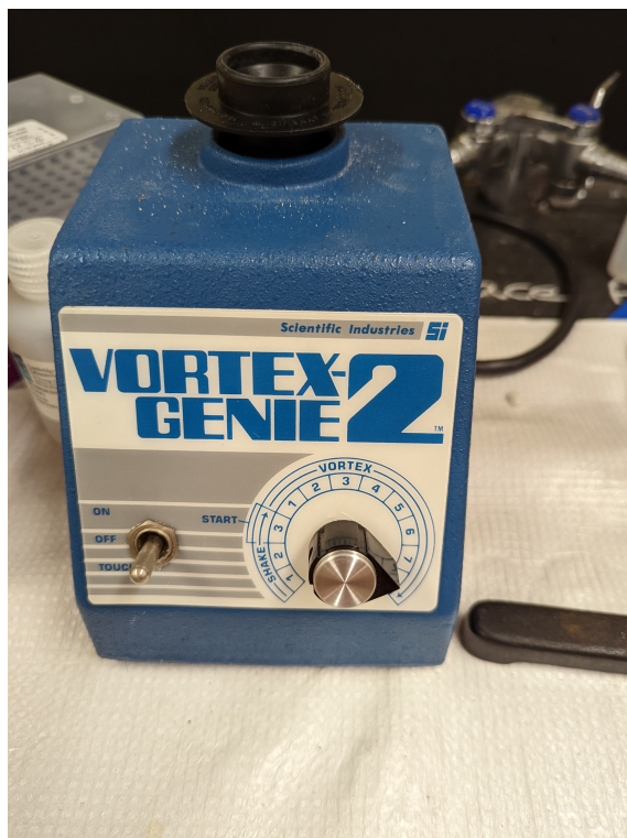
Figure 3.7: Vortex Genie from Scientific Industries. Used for initial mixing of solute and solvent.
