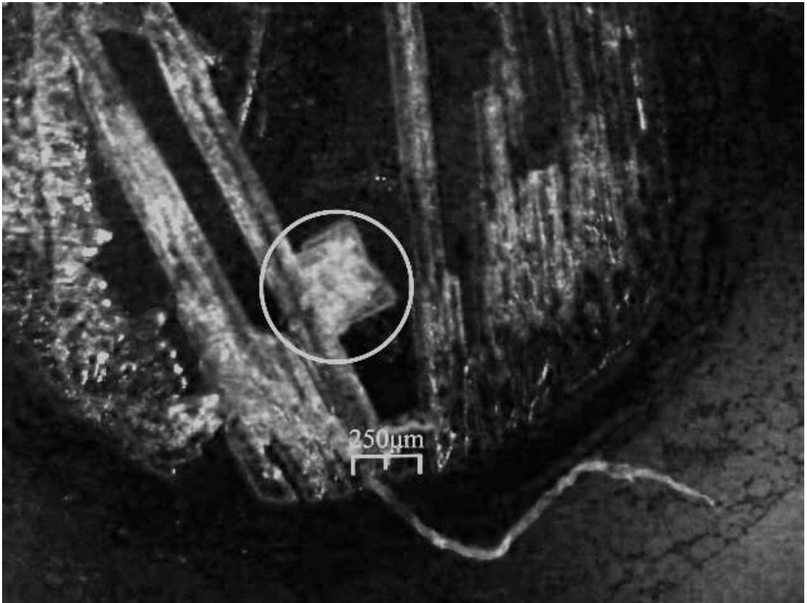
Figure 5.1: Satellite tobacco mosaic virus crystal on a silicon substrate. Crystallized (\text{NH}_4)_2\text{SO}_4 is also seen around the virus crystal. Image taken using Supereyes digital microscope.
