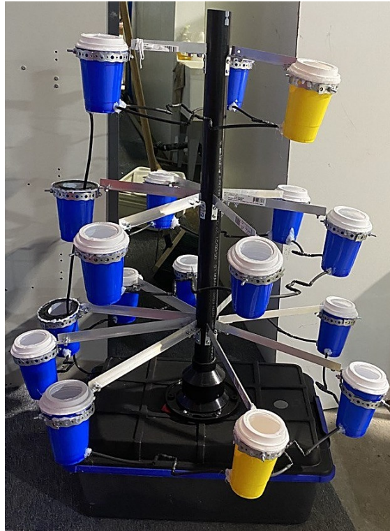
Figure 3.6: The constructed initial prototype of the C-Tree hydroponic system
