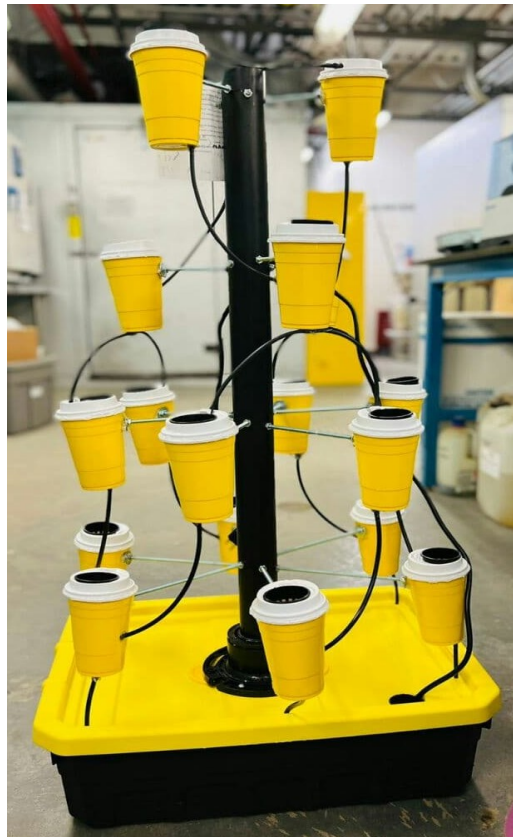
Figure 3.12: The final constructed C-Tree hydroponic system
