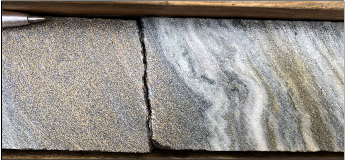
Fig. A1. 14 Exhalative-style barite-rich massive sulfide mineralization in drill hole 109 @ 206 m. Layers of honey-brown sphalerite contain disseminated sulfosalts and alternate with white, barite-rich layers.
