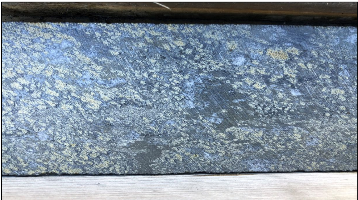
Fig. A1. 15 Replacement-style VMS mineralization in drill hole 110 @ 263.6 m. Blebby honey brown sphalerite and white barite replaced the tuffaceous matrix. Relic lapilli (darker shades) are replaced by very fine-grained sericite and pyrite.
