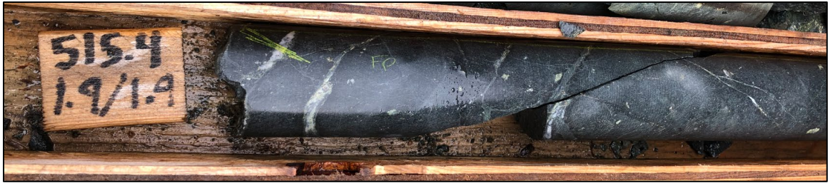
Fig. A1. 7 Drill core photograph of ferroandesite (FeA) with sparse feldspar phenocrysts. Sample W813093 in drill hole 112 @ 515.4 m.
