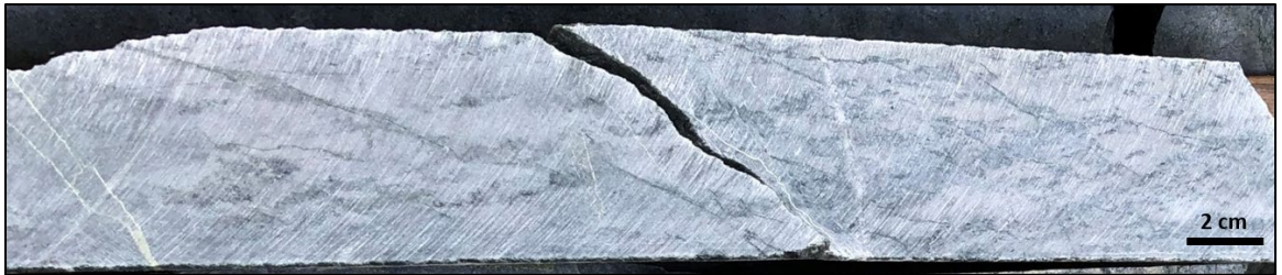
Fig. A5. 2 Sample 110-368 of massive FIIIb high-silica rhyolite (HSR) with patchy epidote, calcite, and chlorite alteration.
