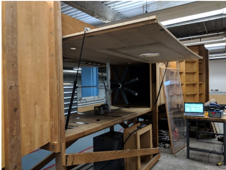
Figure 20 - Image showing open sides of wind tunnel setup.
