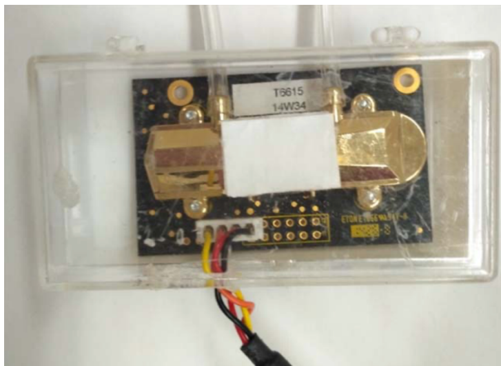
Figure 2.4. The NDIR CO 2 sensor.
