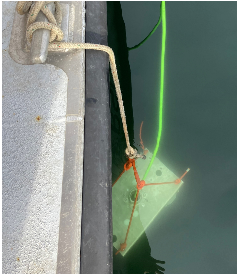
Figure 5.8: Airmar M475 transducer hanging on the side of the vessel, photo from the February 1, 2023, field trip.
