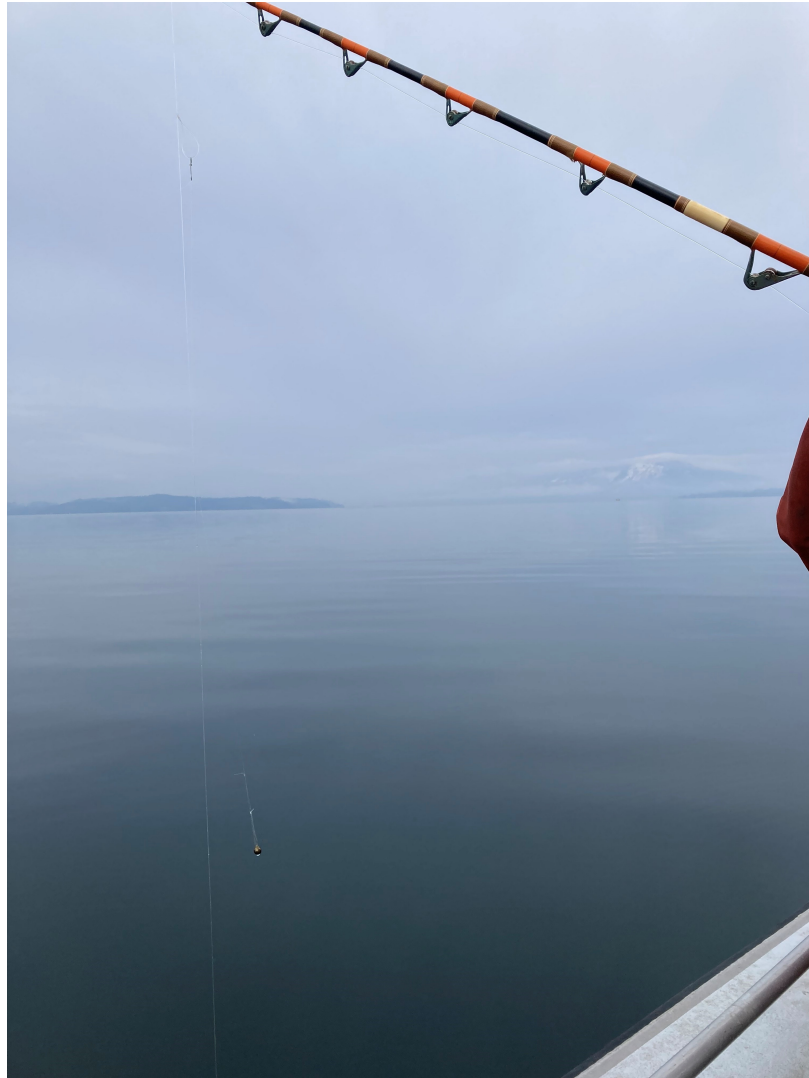
Figure 5.9: Tungsten calibration sphere attached to the fishing line, photo from the February 1, 2023, field trip.
