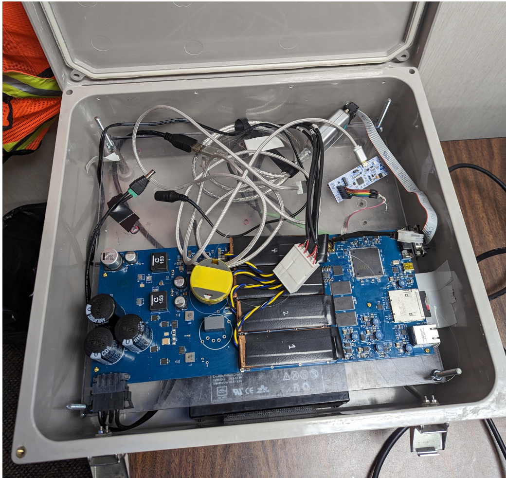
Figure 5.2: AZFP-Split prototype circuit board during the field trials. The battery is under the board.
