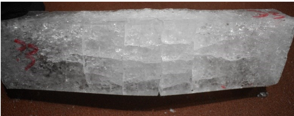
Figure 4-17 – Sample that did not fail completely for 135% compression and low speed. (a.) side view of the sample; (b.) top view; and (c.) bottom view.
