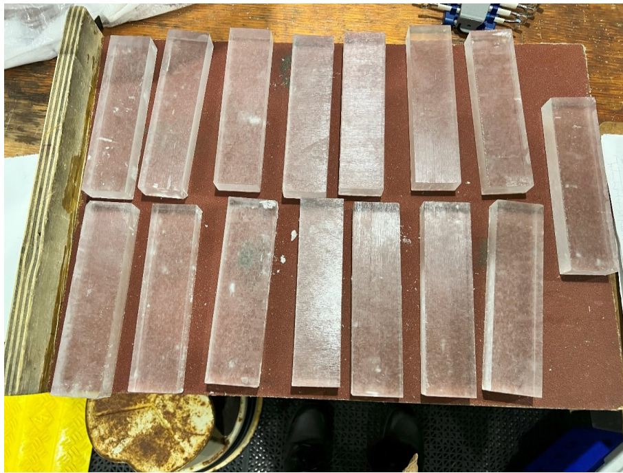
Figure 3-3 – Ice beams cut out of polycrystalline ice block made using the vacuum mold method.
