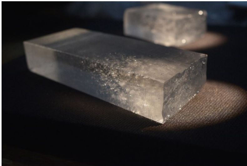
Figure 4-15 – Fracture surface of ice beam in simple flexural loading.
