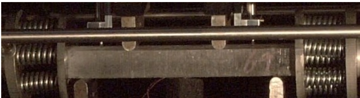
Figure 3-16 – Ice sample preloaded by indenters and axially loaded by plates and springs.
