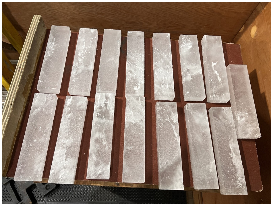
Figure 3-9 – Saline ice prisms prepared for flexural testing.
