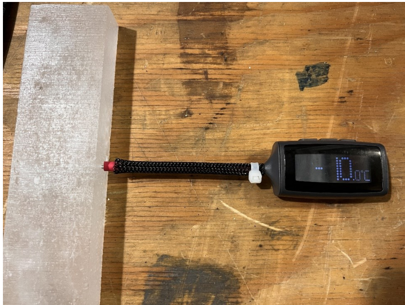
Figure 3-11 – Centrepoint temperature of the sample before moving to -10 °C room (a.) and temperature stabilized to -10 °C (b.)
