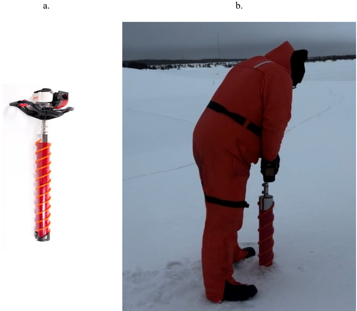
Figure 3-6 – (a.) Kovacs ice corer; and (b.) corer being drilled into the ice sheet.
