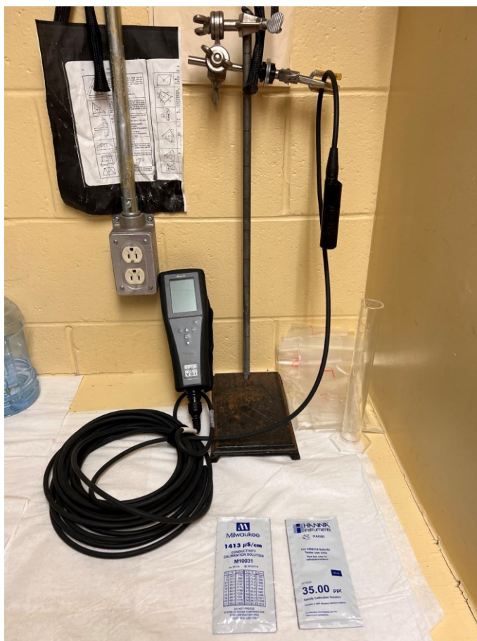
Figure 3-12 – Salinity measurement device connected to probe via a cable. The calibration solutions graduated cylinder and melted saline ice samples are also shown.
