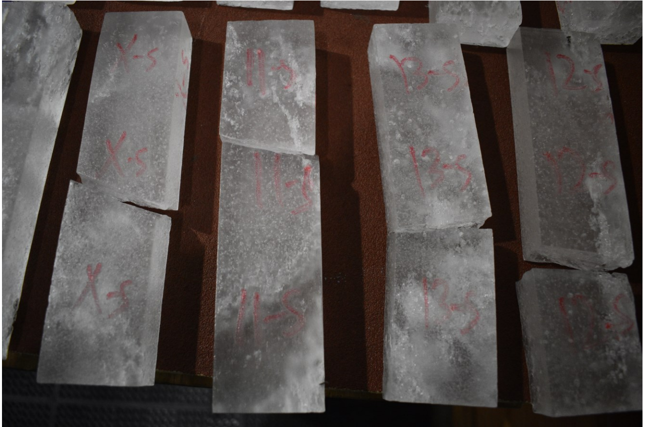
Figure 5-18 - Saline ice samples tested in 4-point bending tests.
