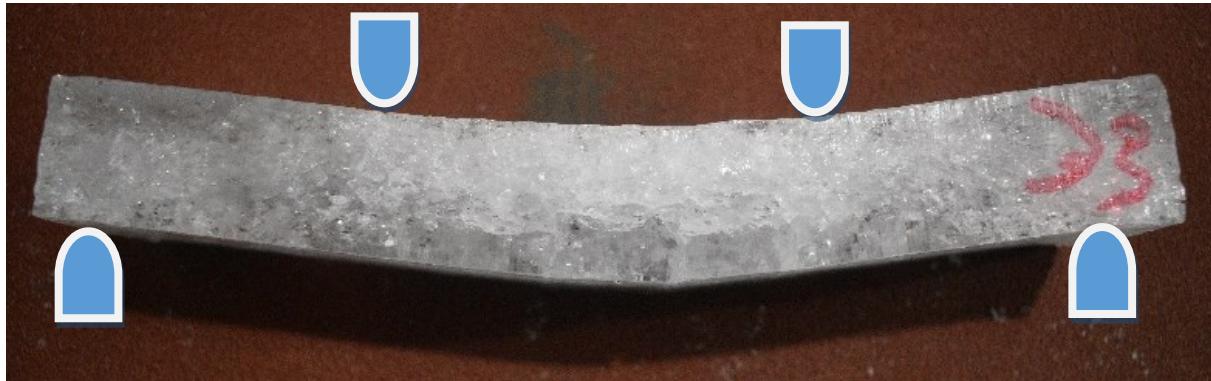
Figure 4-18 – Ice sample with approximate indenter locations.
