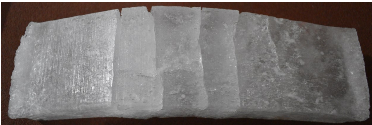
Figure 5-25 - Tensile cracks of a partially failed sample.
