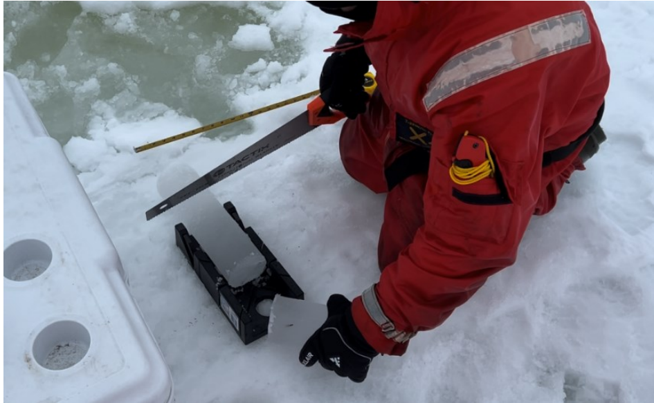
Figure 3-7 – Cores cut into smaller sections that can fit inside the cooler using a handsaw.
