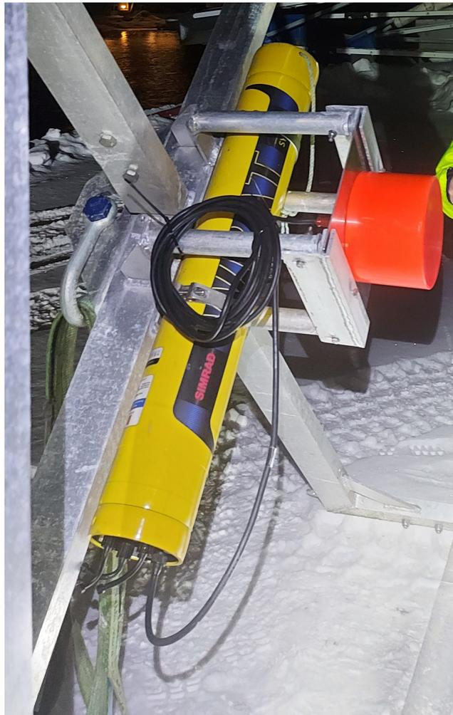
Figure 1.1: Image of a wideband autonomous transceiver (yellow cylinder; Kongsberg Discovery AS, Horten, Norway) with a 38 kHz split-beam transducer (orange). Photo taken by Stig Falk-Petersen.
