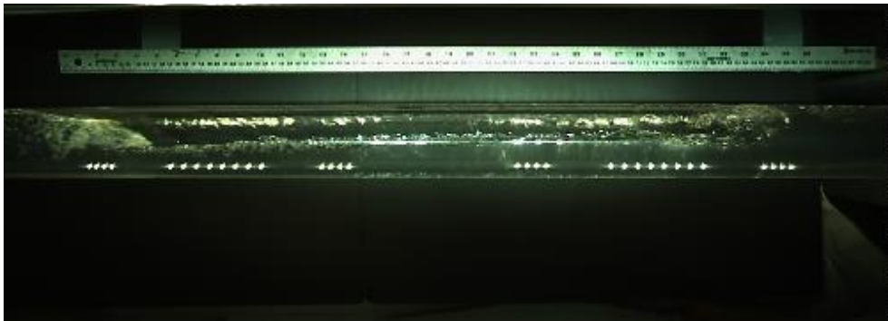
Figure C.4: Flow patterns air-water two-phase flow – slug flow
