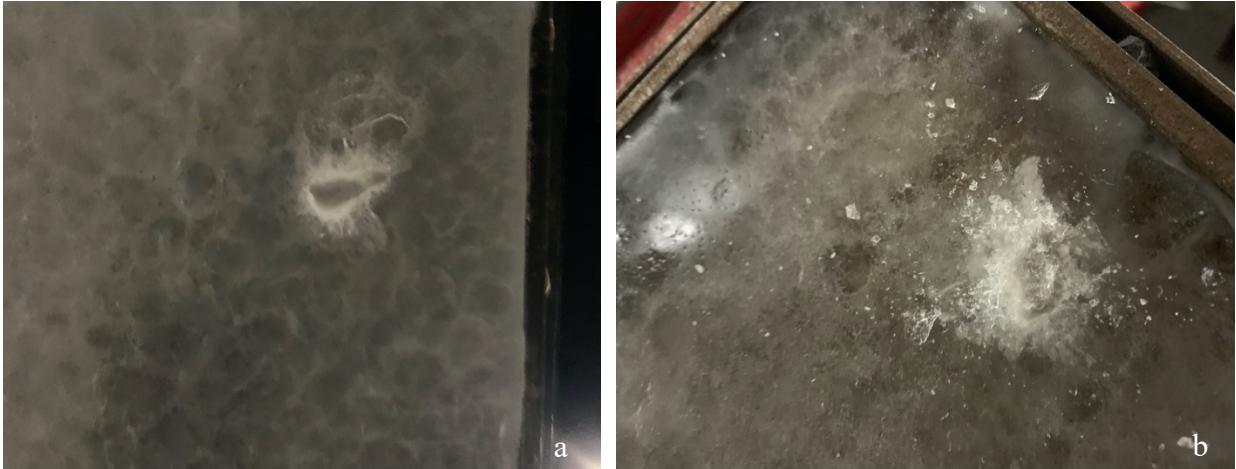
Figure 28 – Images taken after indentation of upper ice specimen (a) and lower ice specimen (b).
