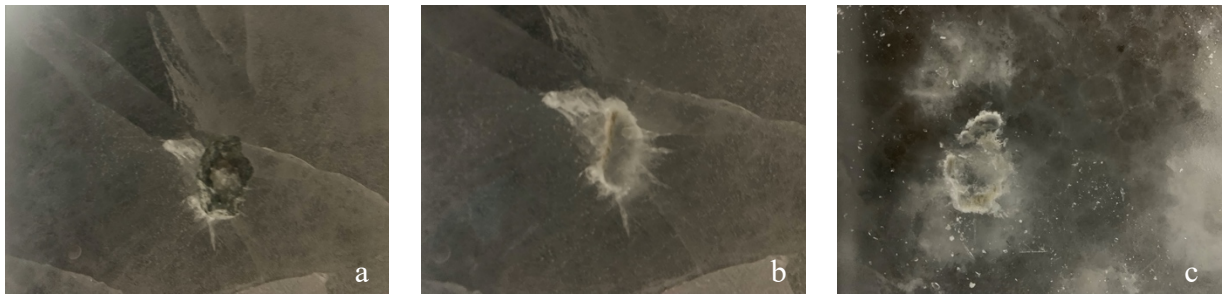
Figure 25 – Images taken after indentation of upper ice specimen (a)(b) and lower ice specimen (c).
