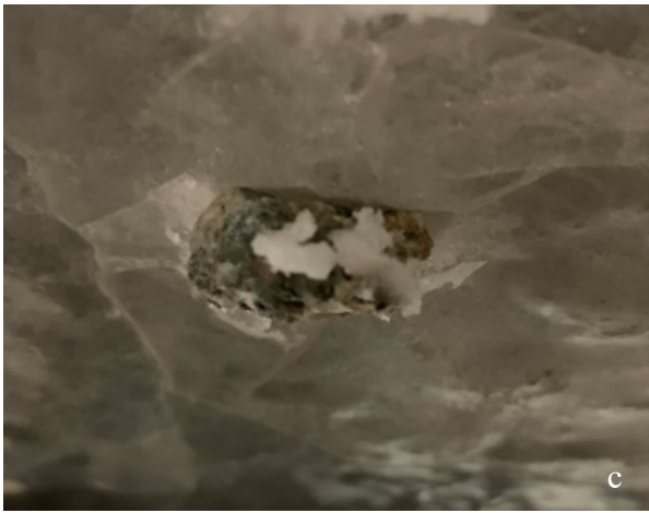
Figure 63 - Images of bottom (left) and top (right) ice surfaces taken after testing for 7D (a./b.) and 2D (c./d.).
