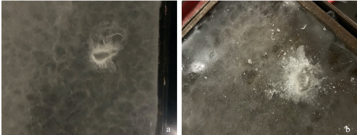
Figure 34 - Images taken after indentation of upper ice specimen (a) and lower ice specimen (b).
