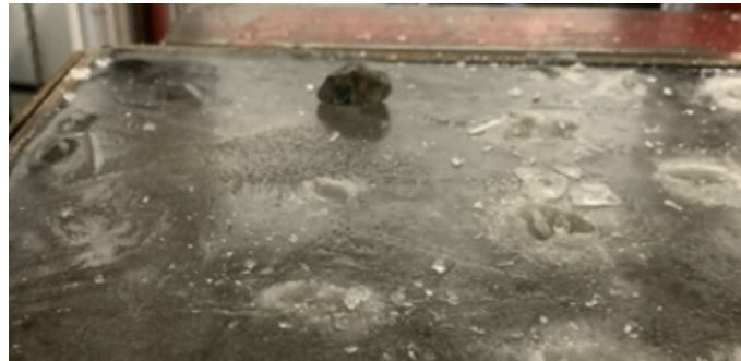
Figure 53 – Image taken before testing showing rock placement relative to prior test indentation locations.
