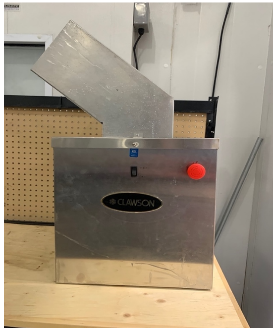
Figure 19 – Ice crusher used to create ice seed.
