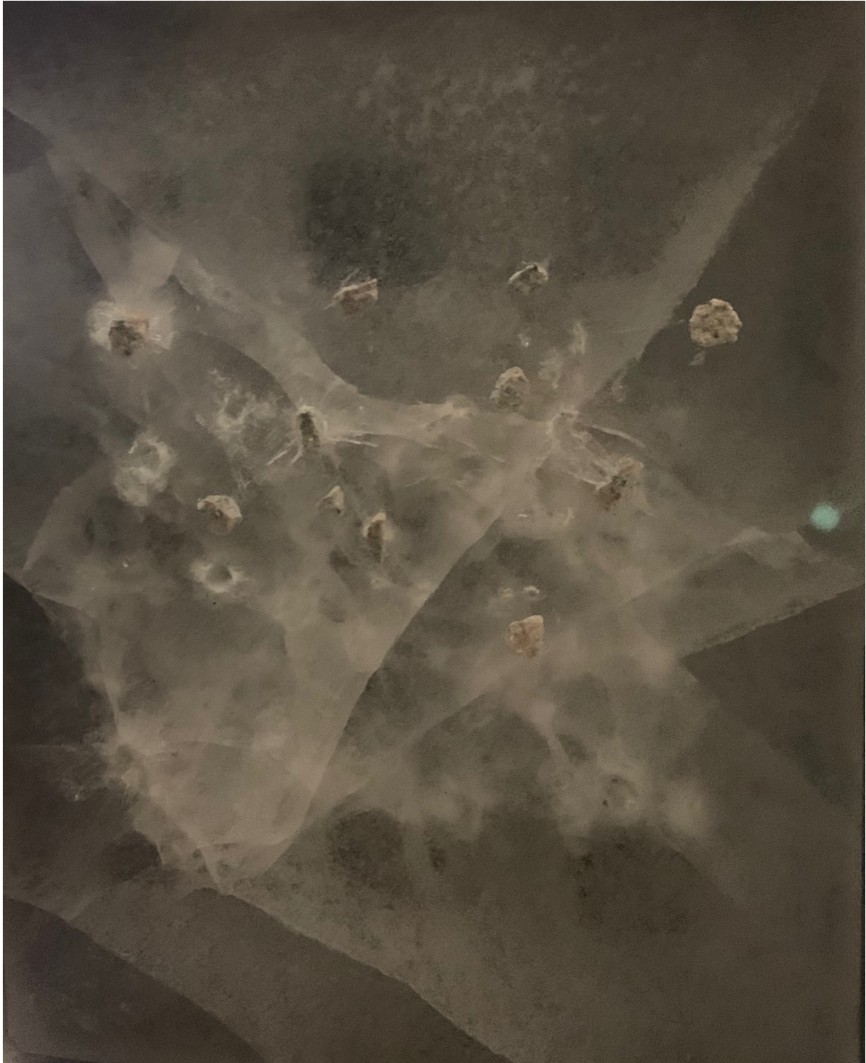
Figure 42 - Image taken after indentation of upper ice specimen, 5mm indentation.
