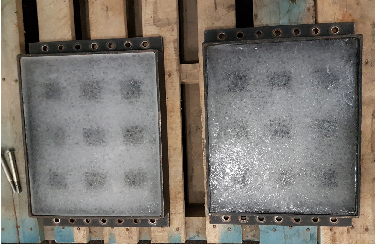
Figure 18 – Upper ice specimen, frozen in ice mold before being affixed to horizontal carriage
