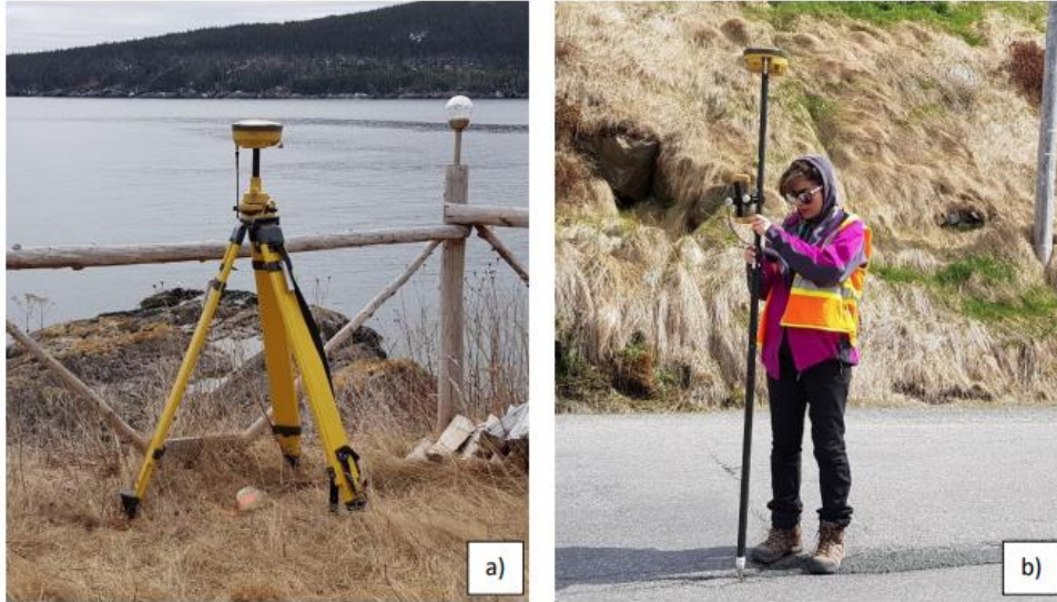
Figure 3-31) a) RTK base receiver on a tripod. Bread and Cheese site, April 1, 2021. b) RTK rover receiver on staff. Operator Marzieh Arshian. The Cliff site, April 26, 2021.
