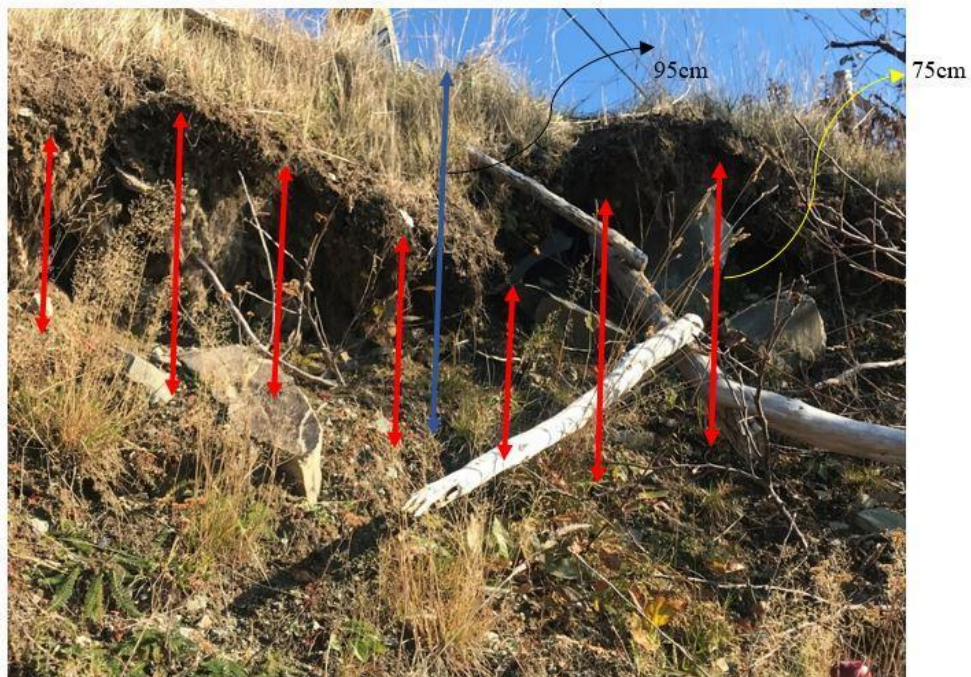
Figure 2-12) An expanded view of separations shown in Figure 2-11. Average amount of separation was 50 cm and the distance from the top of the bank was roughly 95cm.
