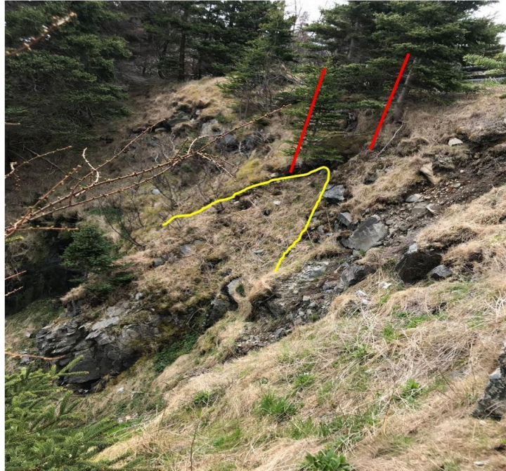
Figure 2-32) The yellow curve shows the soil creeping area (failure of soil cohesion), and the red line depicts that the tree is not straight yet. (Quays site, first eastern inlet.)
