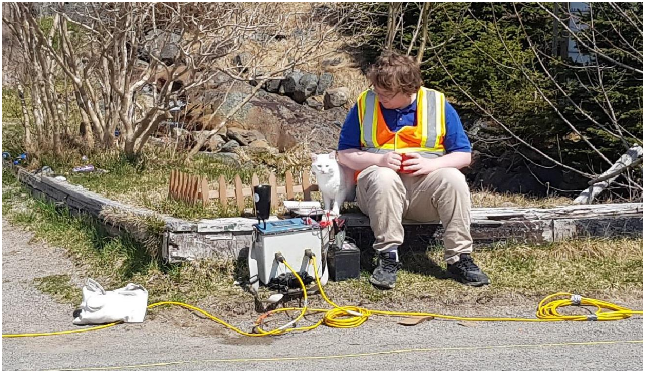
Figure 4-2) Illustrates the programmable Iris Instruments Syscal Junior DCR unit used to collect data in Bay Bulls. The control and storage unit was located in the middle of the spread.
