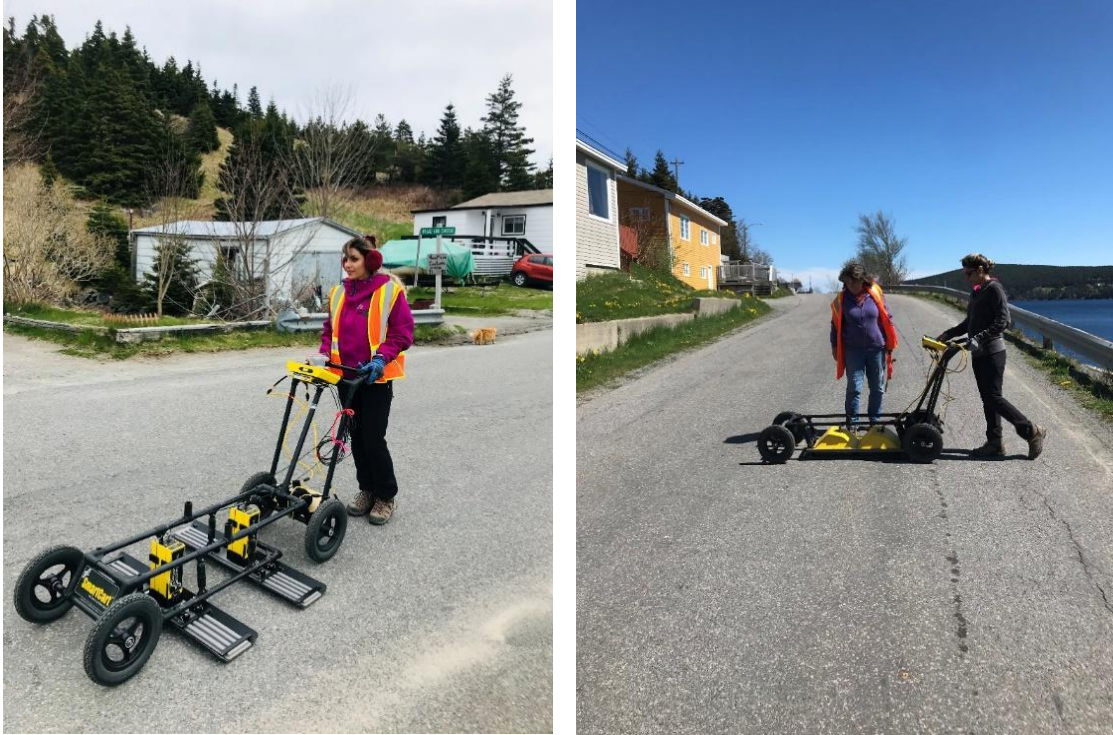
Figure 4-5) Sensors & Software EKKO Pulse Pro GPR with (a) 100 and (b) 250 MHz antennas. Operated by Marzieh Arshian. The two yellow mounds in (b) are shields covering the transmitter (back) and receiver (front) antennas. A skid plate separates the antennas from the road.
