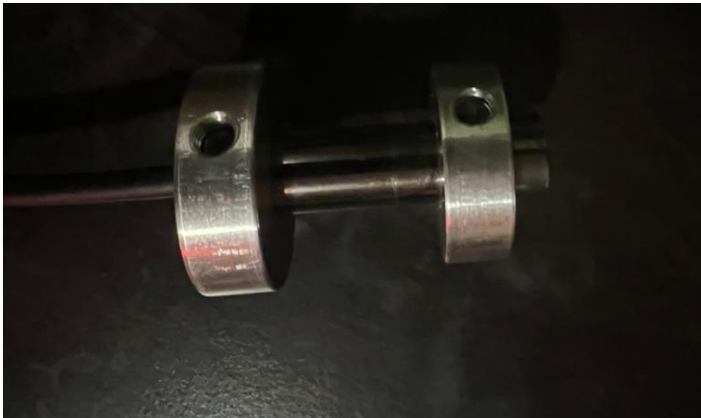
Figure 19 – Borescope camera with two set screw collars attached.
