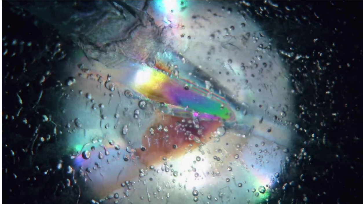
Figure 71 – Bubbles present at the surface of an ice sample prior to testing – Test 7.
