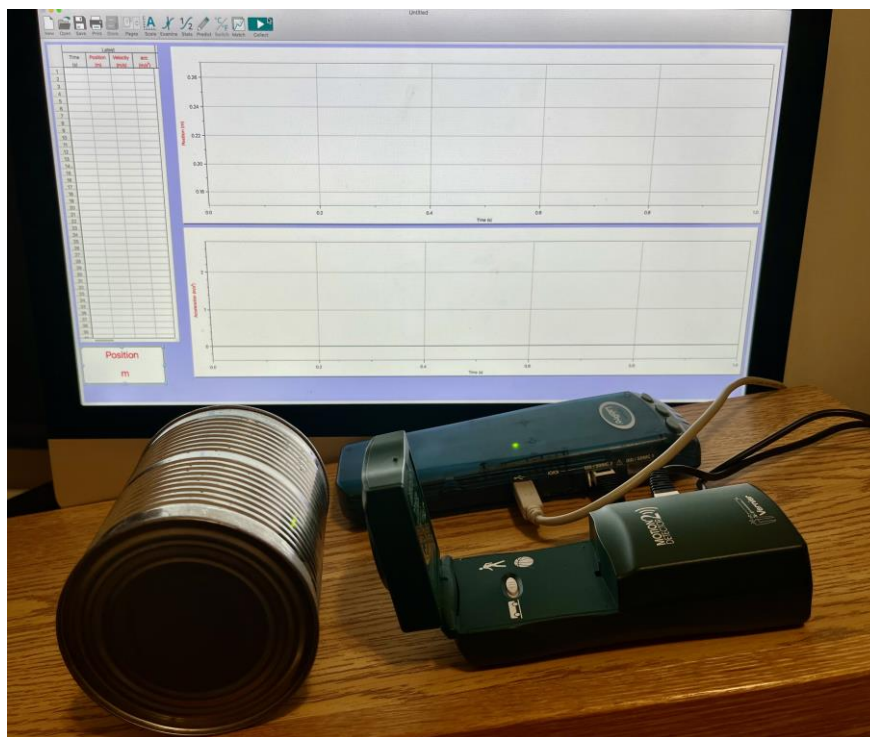
Figure 2. Apparatus for Motion on an Inclined Plane Inquiry. This apparatus for motion on an inclined plane inquiry that was used to measure the velocity of the can as it moved down the ramp away from the motion sensor (both in the foreground). The LabPro interface and monitor are in the background with the data collection software. As the can moved down the ramp (see Figure 5), a graph of motion was instantaneously produced.
