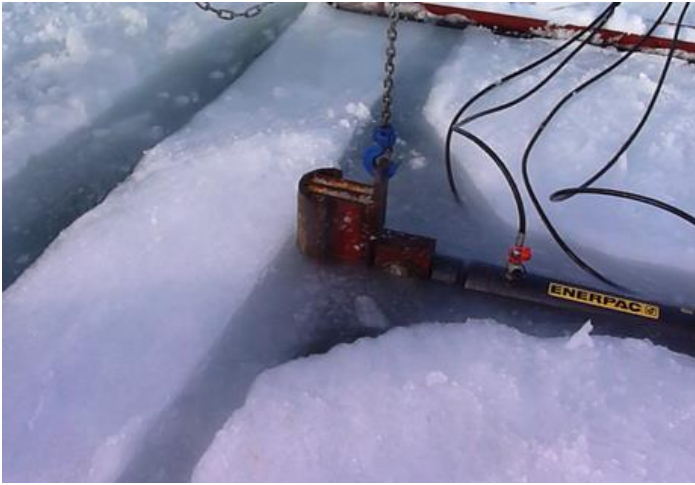
Figure 4-2. Photos of: (left) the beam test setup; (right) failed beam specimen
