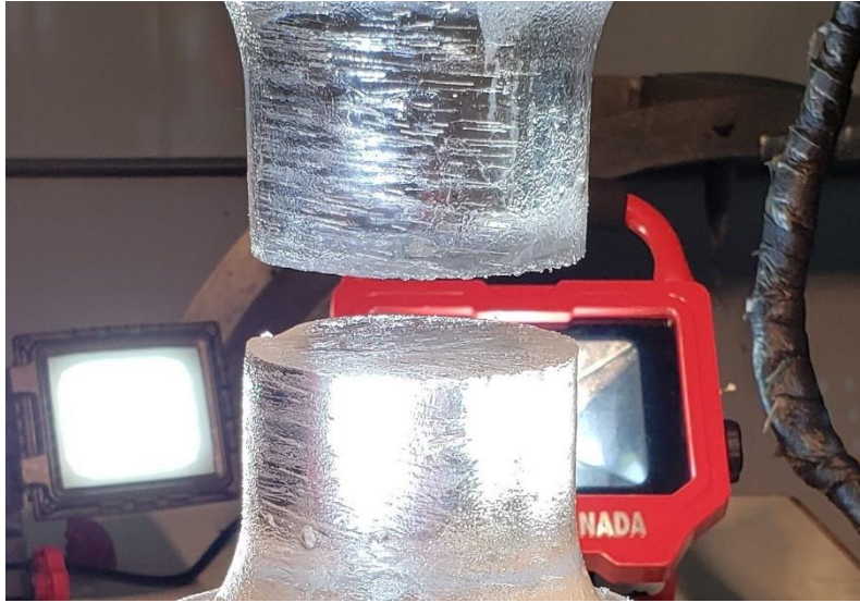
Figure 3-6- Photo of a reduced (dumbbell shape) sample after failure
