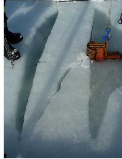
Figure 4-2. Photos of: (left) the beam test setup; (right) failed beam specimen
