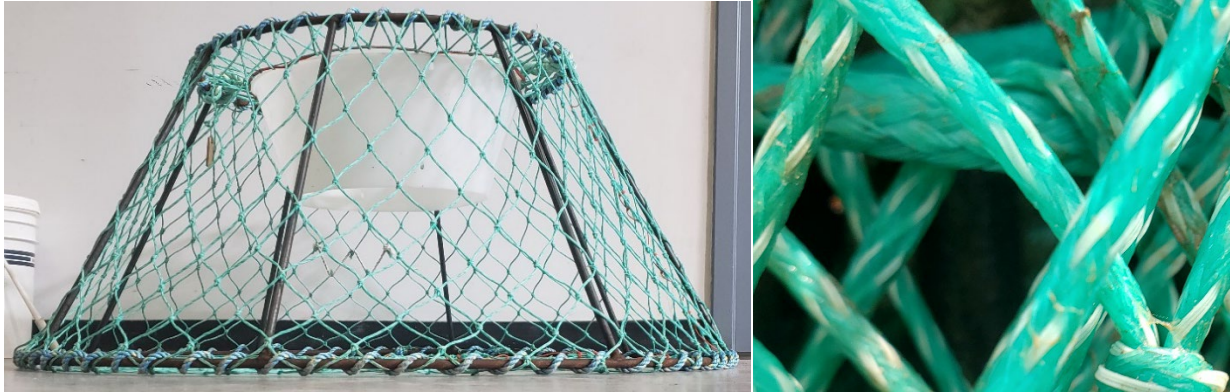
Figure 3.1 Image on the left is a luminescent-netting snow crab pot used in the Newfoundland and Labrador snow crab fishery. Image on the right is a close view of the netting (6-strand) of a stack of the same pots.
