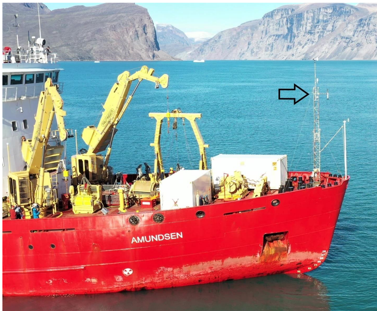
Figure 30: The measurement tower at the bow of the ship with anemometer, temperature sensor, and air inlet mounted on the truss approximately where the arrow is pointing. The GPS was fixed at the lower end of the truss. Photo credit to David Cote (DFO, Canada).
