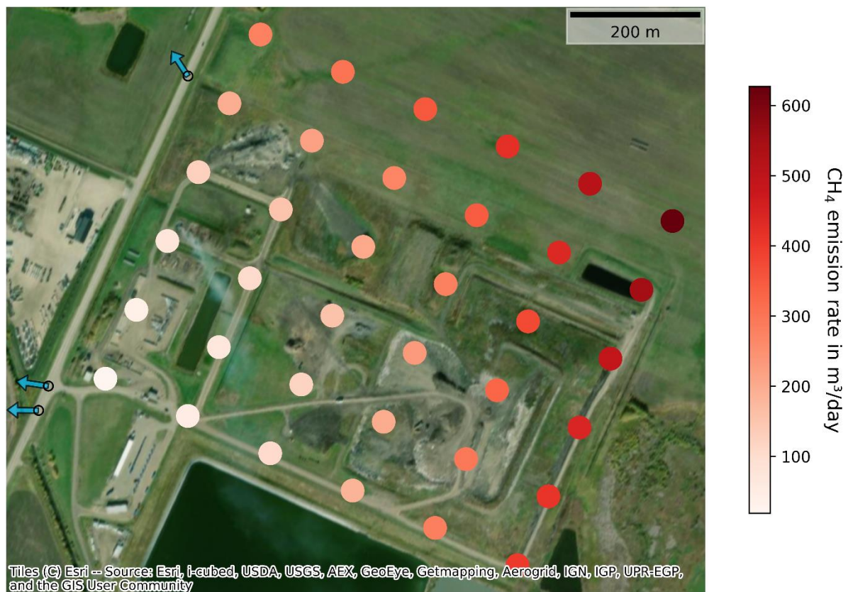
Figure 27: Point-level emission rates within the landfill terrain in Grande Prairie. The black circles on the road represent the points during the truck survey when CH 4 peaks were detected downwind of the landfill on three different passes on two days. Blue arrows indicate the direction the wind is blowing to at the time of detection.
