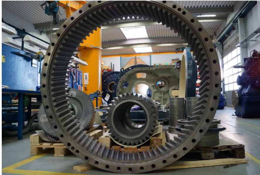
Fig. 1.4 Disassembled ring gear of a wind turbine PGT [11]
