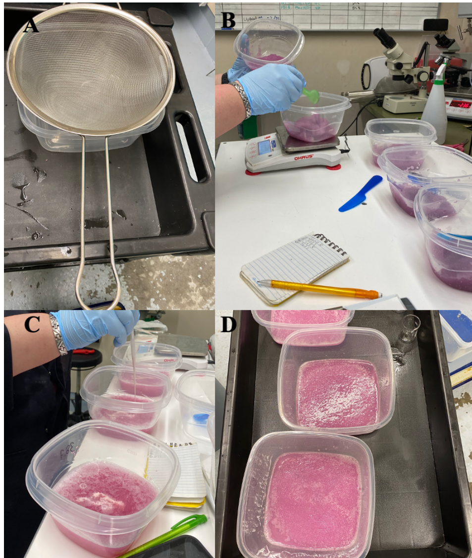
Figure 3.6: Combining of egg masses from 3 different female lumpfish and fertilizing them with milt from 2 different male lumpfish. The eggs and ovarian fluid from each female were separated using a fresh container and a strainer (A). The ‘dry’ egg masses were then weighed, and 80 g of eggs from each female were combined to produce 3 new egg masses (B). The ovarian fluid (1/3 rd from each female) was then added to the ‘dry’ egg masses, and each egg mass was fertilized with 3 mL of milt, 1.5 mL from each of 2 males (C). Lastly, the egg masses were stirred, and poured into new containers (D) prior to being placed in the incubators.
