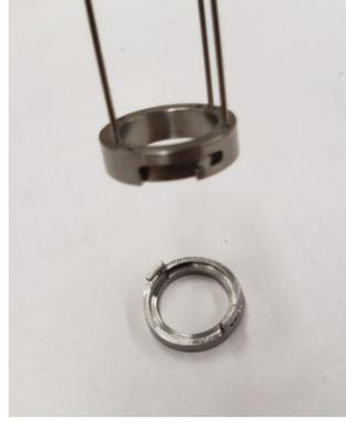
(b) Fabricated reactor bed
